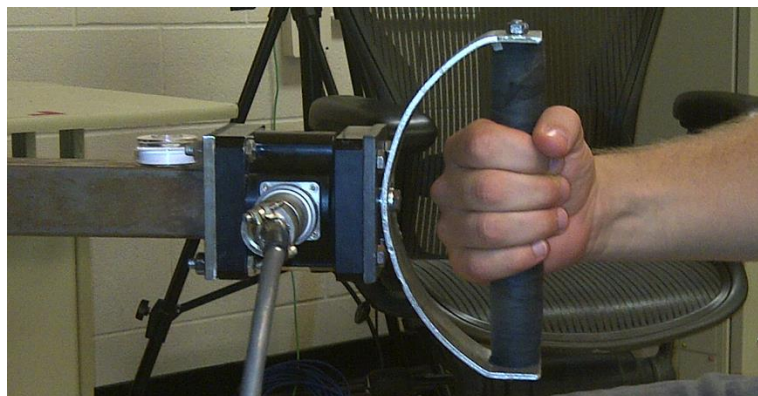
Figure 3.3 Force handle attachment for force exertions
