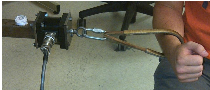
Figure 3.2 Leather strap attachment for joint moment capacity testing
