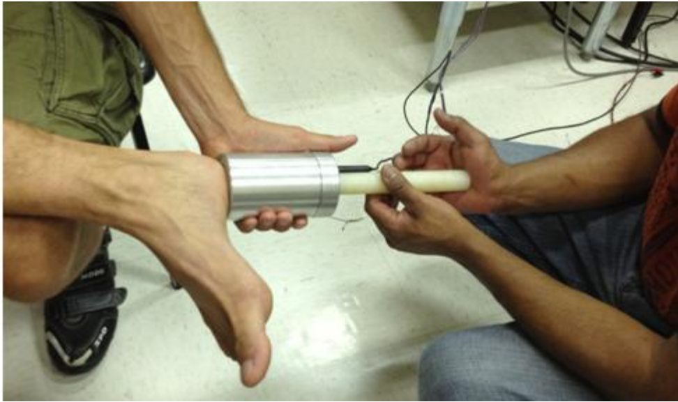
Figure 2.18: Force Displacement sensor applied to plantar heel soft tissue
