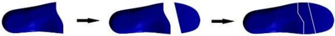
Figure 4.5: First the posterior FO surface is designed, then the anterior FO surface, and finally the model is completed by adding the transition FO surface
