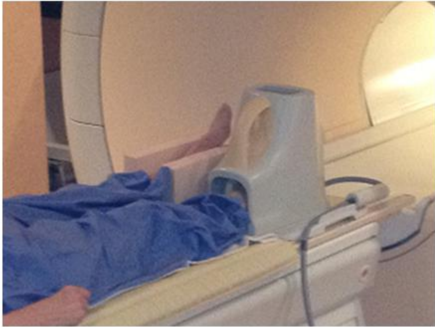
Figure 2.2: MRI scanning the foot with a fixture for both housing a dedicated coil and restraining the foot
