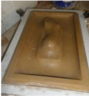
Figure 1.13: Creating the FO shell by vacuum forming materials to the positive cast
