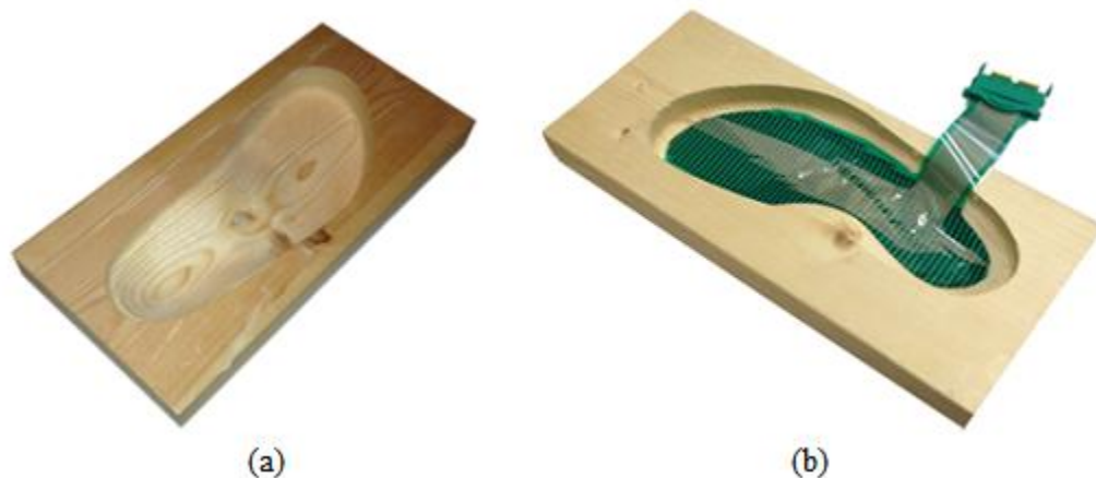
Figure 2.22: a) Machined FO surface, b) F-Scan sensor under trimmed and taped to the FO surface to minimize kinking
