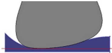
Figure 4.9: An end angle of 0 is advisable for the arch region of the foot
