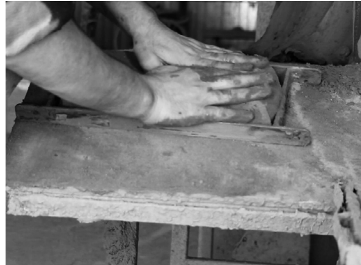
2.2. At Fornace Bernasconi in Castel Viscardo, Italy, each brick is hand-formed in a metal mold. 2.3. (opposite) The fired bricks.
