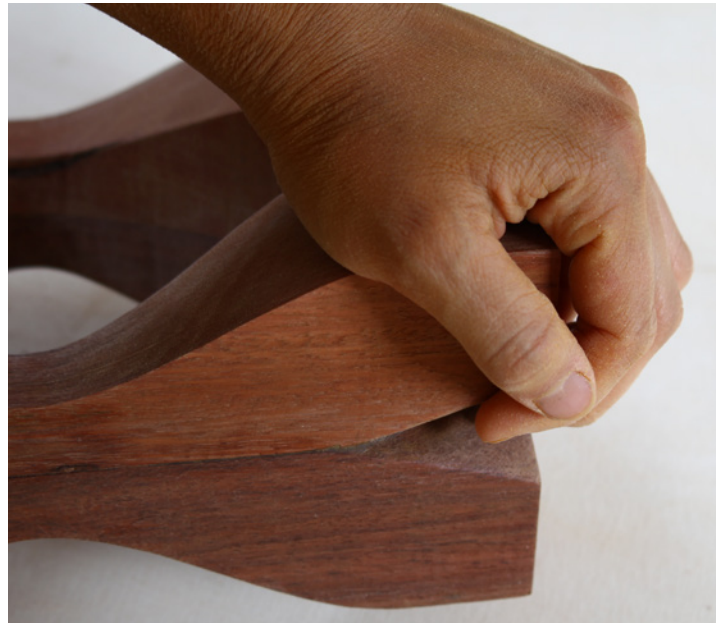
2.13. The first mold was fabricated in two pieces using the CNC router and subsequently assembled.
