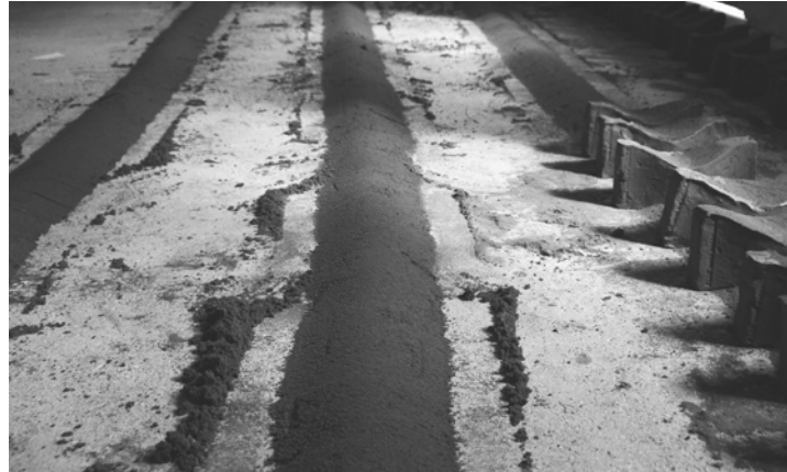
2.20. The rows of sand support the drying bricks from underneath.
