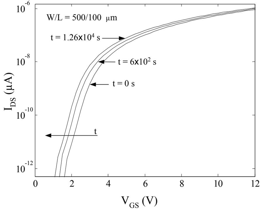
**Fig. 4.2 I-V characteristics of a TFT plotted on a semi-logarithmic scale after  $t = 0$ ,  $6 \times 10^2$ , and  $1.26 \times 10^4$  seconds of removing the 20V gate bias stress.**
