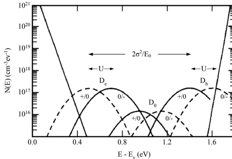
**Fig. 3.8** Calculated density of states (DOS) in a-Si:H.  $D_e$ ,  $D_h$ , and  $D_0$  states and their corresponding  $+/0$  and  $0/-$  transitions are shown; the valence and conduction band tails are also indicated [54].
