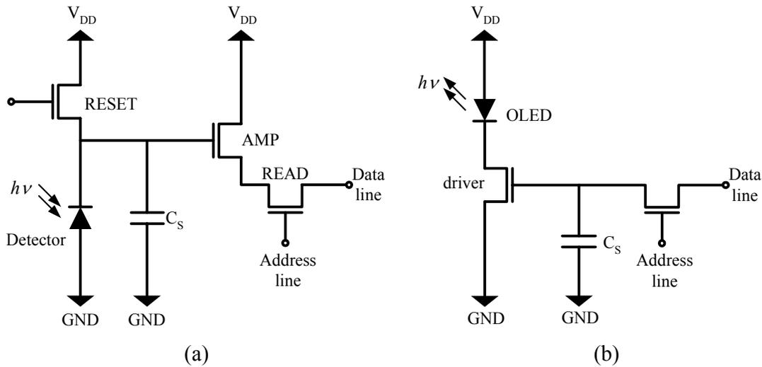
**Fig. 2.4 Pixel architecture for (a) an APS and (b) an AMOLED display.**
