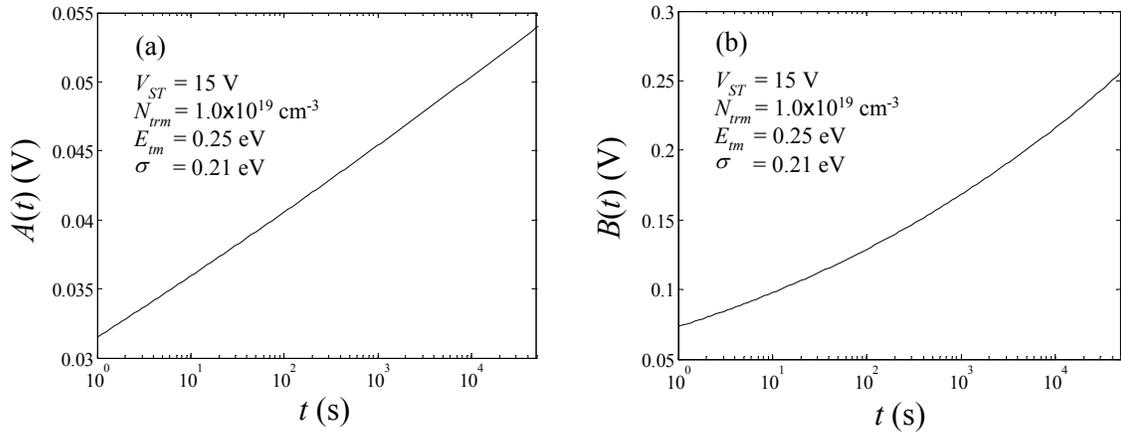
**Fig. 3.14** Calculated (a)  $A(t)$  and (b)  $B(t)$  using (3.50) and (3.51), respectively, for a 15V bias stress.
