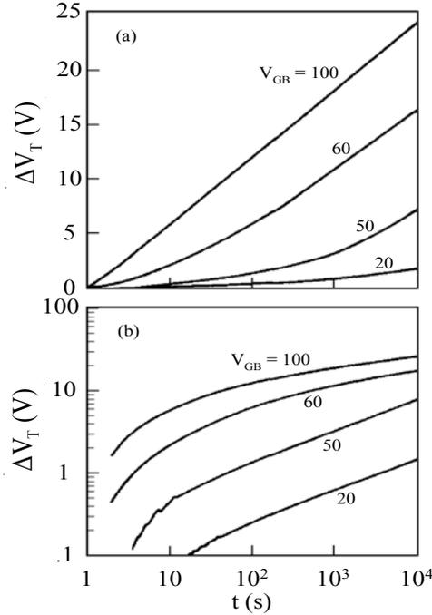
**Fig. 3.9 Threshold voltage shift versus time for different stress voltages plotted on (a) a linear scale and (b) a logarithmic scale [51].**
