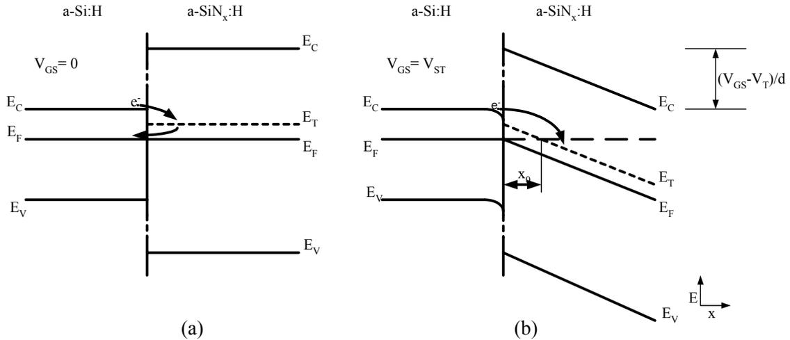
**Fig. 3.10 Energy-band diagram of the a-Si:H TFT near the gate dielectric interface for (a)  $V_{GS} = 0$  and (b)  $V_{GS} = V_{ST}$ .**
