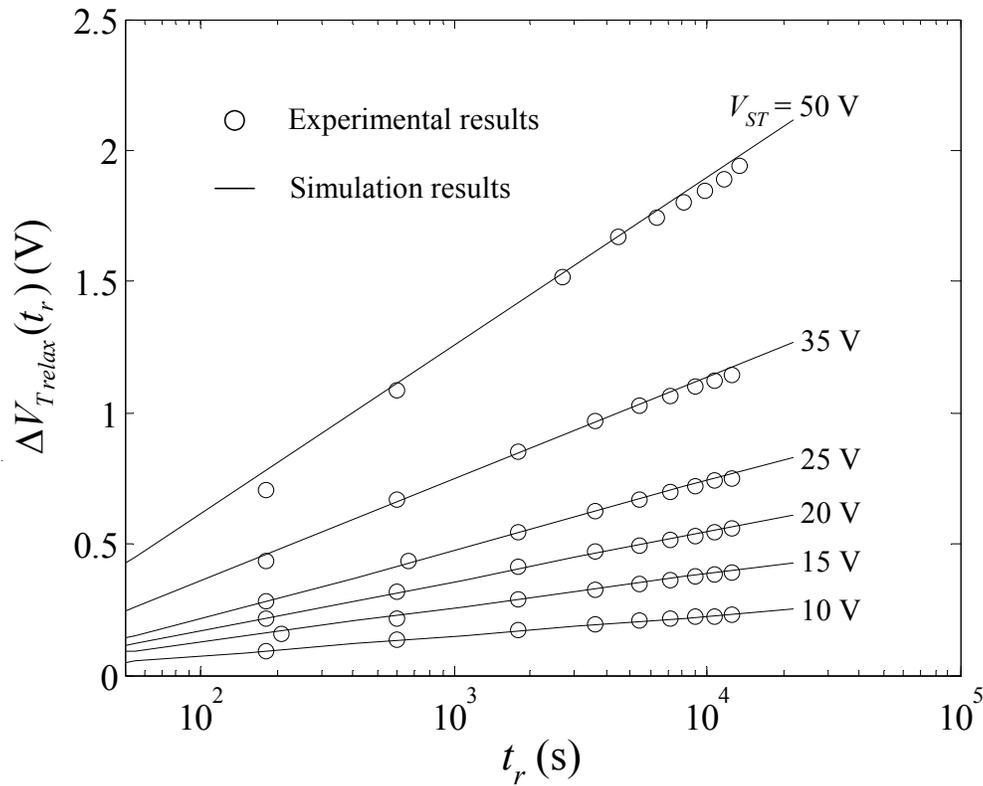
**Fig. 4.7 Charge de-trapping simulation results using the parameters of Table 4.2 after 3.5 hours of bias stress with  $V_{ST}$ ; the experimental results are also shown (open circles).**
