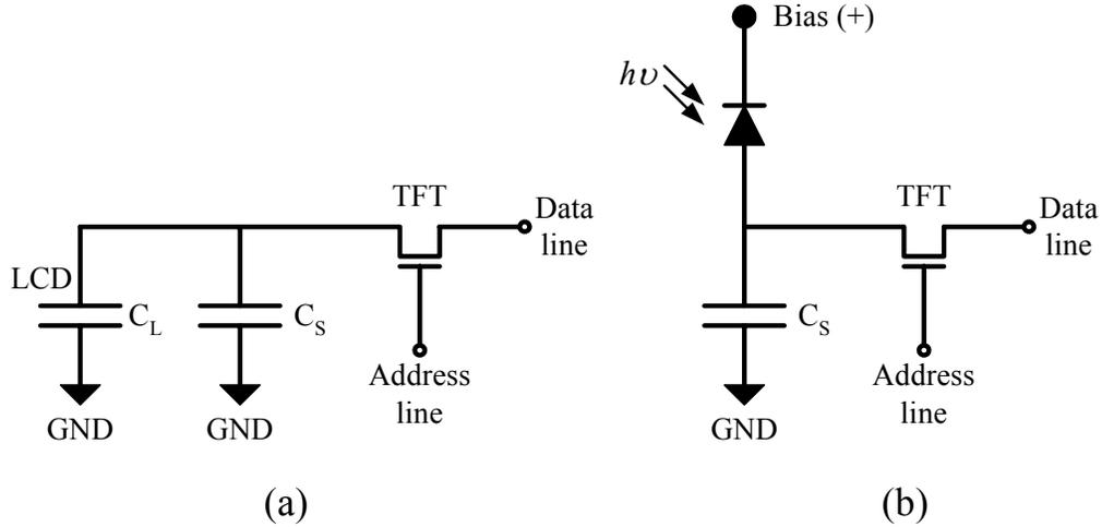
**Fig. 2.3 Pixel architecture for (a) an AMLCD and (b) a PPS imager.**
