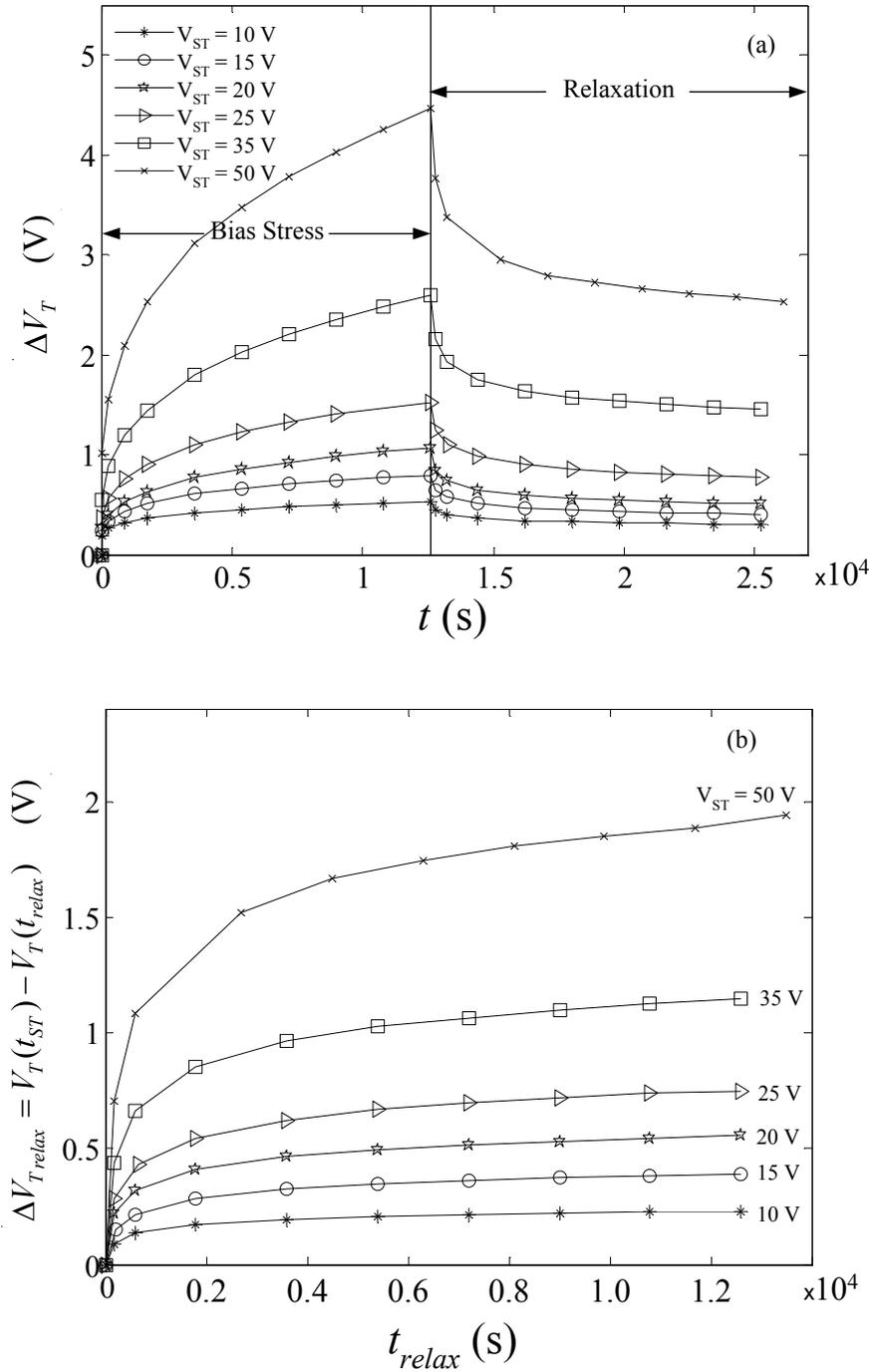
**Fig. 4.3 (a) Threshold voltage shift as a function of time for different bias stresses and (b) relaxation of threshold voltage after 3.5 hours of bias stress at different gate voltages.**
