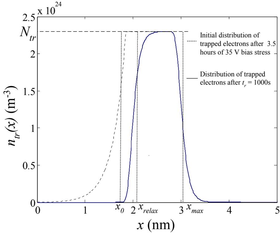
**Fig. 4.8 Distributions of the trapped electrons immediately after a bias stress with 35V for 3.5 hours (dashed lines) and after 100s of relaxation (solid lines); the position of  $x_0$ ,  $x_{max}$ , and  $x_{relax}$  are also shown.**
