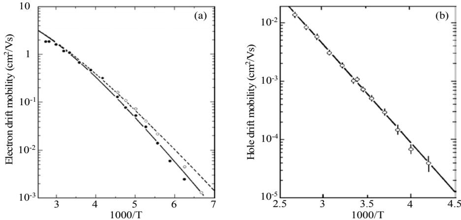
**Fig. 1.4 (a) Electron drift mobility data for an electric field of  $10^4$  V/cm (closed circles) and  $2 \times 10^4$  V/cm (open circles) and (b) hole drift mobility data for an electric field of  $5.8 \times 10^4$  V/cm fitted (lines) to the multiple trapping transport mechanism, assuming exponential band tails [12].**
