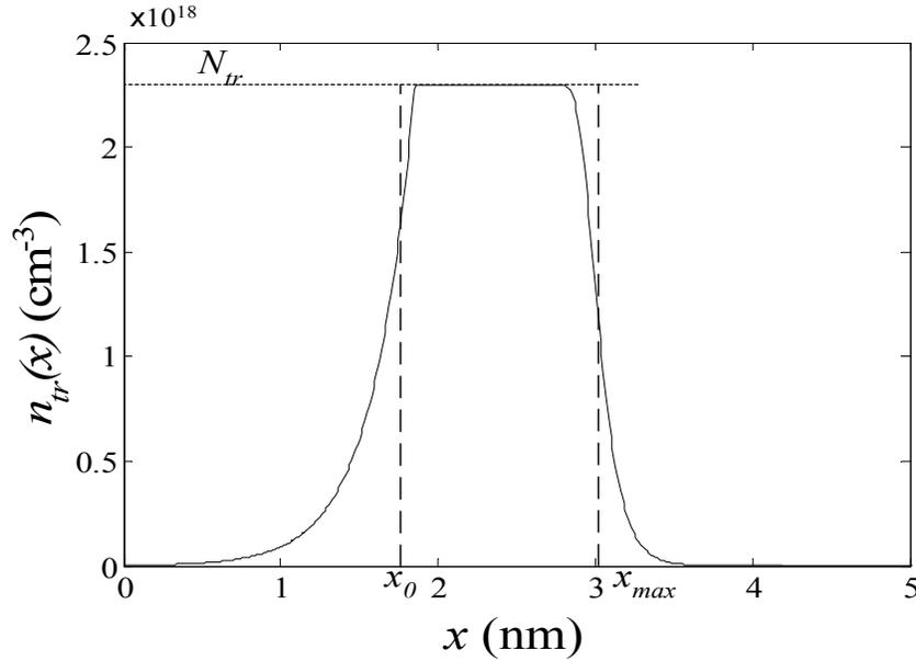
**Fig. 3.11 Calculated trapped electron concentration in SiN as a function of the distance from the a-Si:H/a-SiN<sub>x</sub>:H interface after 3.5 hours of a 35V bias stress using the threshold voltage relaxation results of Chapter 4.**
