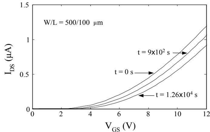
**Fig. 3.2 Transfer characteristics of a TFT at different times after the application of a 20V gate bias stress ( $V_{DS} = 0 \text{ V}$  during the stress).**
