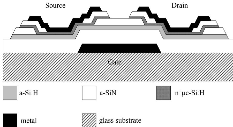
**Fig. 2.1 Schematic cross section of an inverted staggered TFT showing different layers.**
