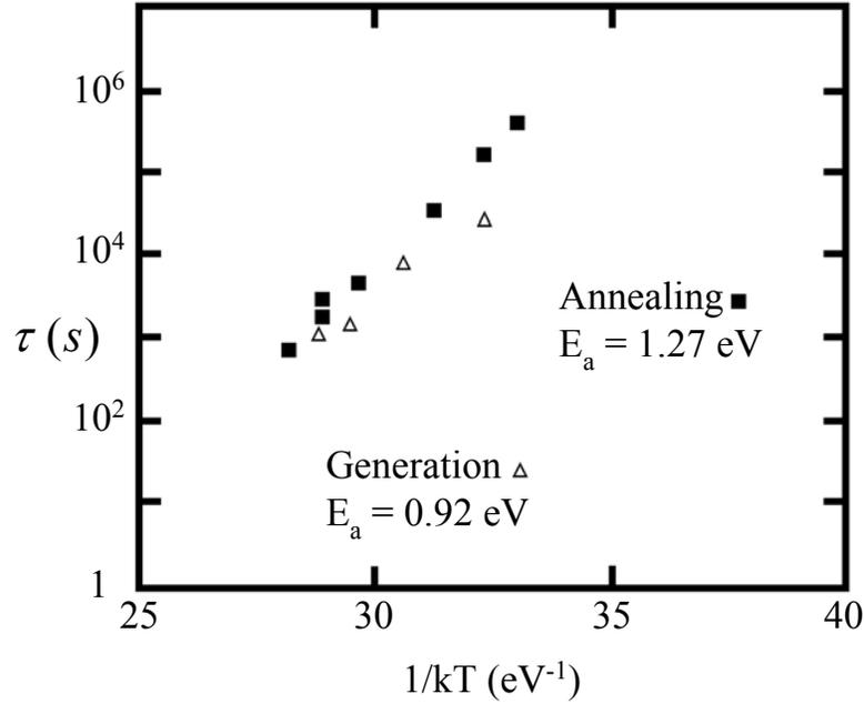
**Fig. 4.5  $\tau$  for the annealing and creation mechanisms as a function of  $1/kT$  [56].**
