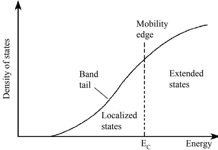
**Fig. 1.2 Density of states (DOS) distribution near the conduction band edge of a-Si:H, showing the localized states and extended states separated by the mobility edge [8].**
