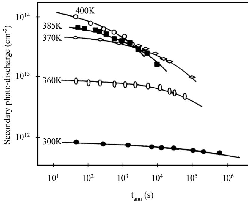
**Fig. 3.6 Secondary photo-discharge response versus annealing time [49].**
