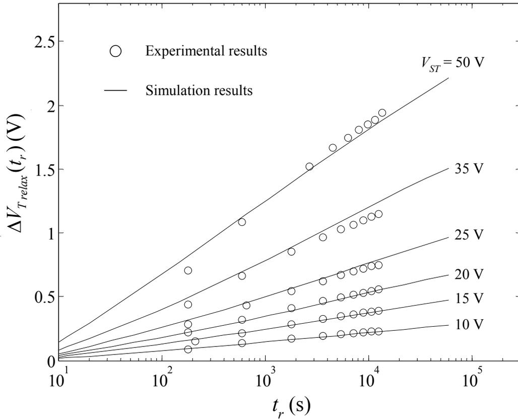
**Fig. 4.12 Calculated threshold voltage relaxation using (4.24) (solid lines) and the experimental results (open circles) after 3.5 hours of bias stress with  $V_{ST}$ .**
