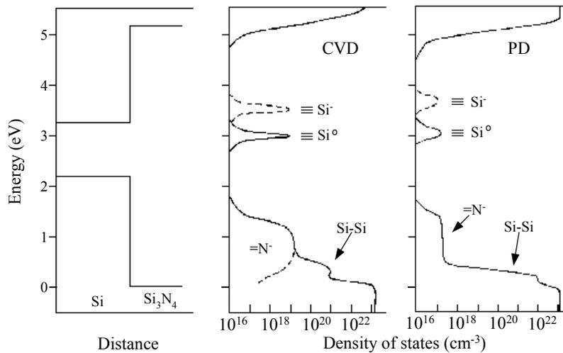
**Fig. 3.12 Proposed density of the gap state for CVD and PD deposited a-SiN<sub>x</sub>:H [68].**
