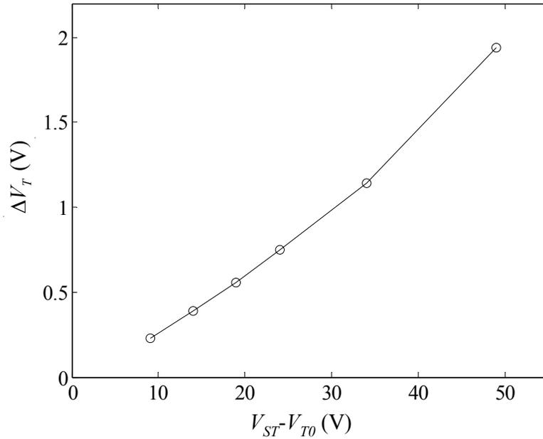
**Fig. 4.4** Threshold voltage relaxation as a function of  $V_{ST} - V_{T0}$  after  $t_{relax} = 1.26 \times 10^4$  seconds of removing the bias stress ( $t_{ST} = t_{relax}$ ).
