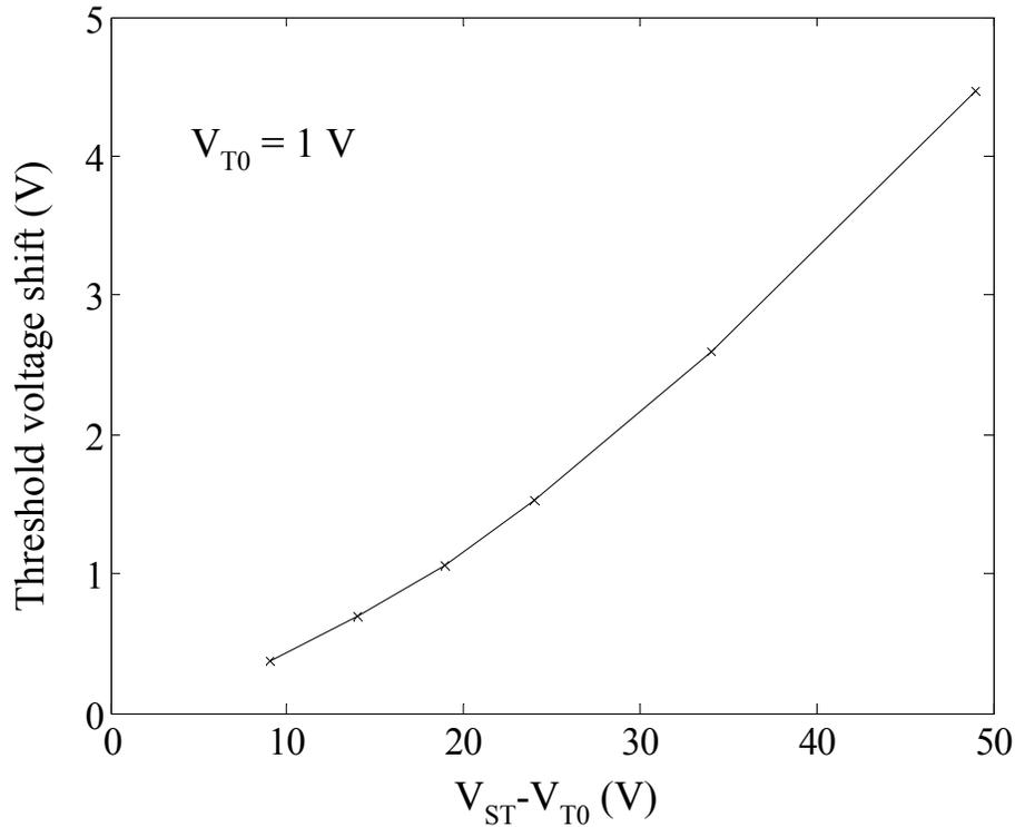
**Fig. 3.5 Threshold voltage shift vs.  $V_{ST} - V_{T0}$  after 3.5 hours of bias stress (during the application of the gate stress  $V_{DS} = 0$  V).**
