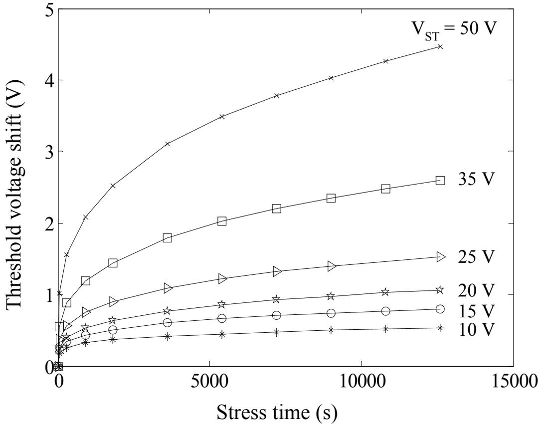
**Fig 3.4 Threshold voltage shift versus time for different stress voltages ( $V_{DS} = 0$  V during the stress, and the TFT aspect ratio is  $W/L = 500/100 \mu\text{m}$ ).**
