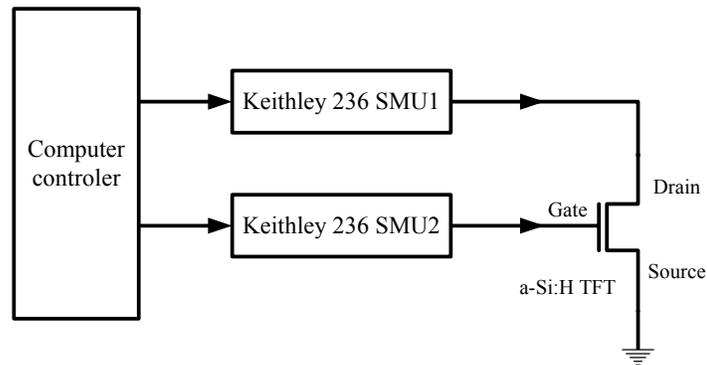
**Fig. 3.1 Experimental setup for the  $\Delta V_T$  measurement.**
