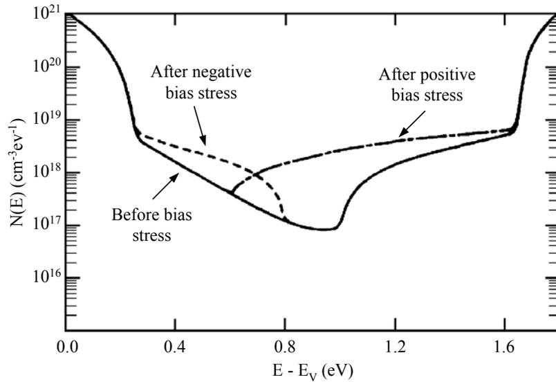
**Fig. 3.7** Calculated density of states (DOS) before (solid line), after positive (chain line), and after negative (dashed line) bias stress for an oxide gate transistor [54].
