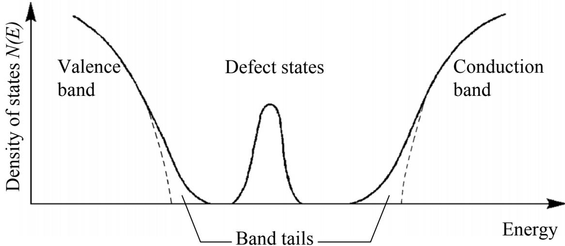
**Fig. 1.1 Schematic density of states (DOS) for a-Si (solid line) and crystalline silicon (dashed lines) showing conduction and valence bands, band tails, and defect states [8].**
