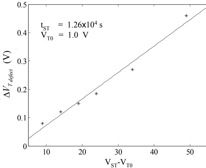
**Fig. 4.14** Calculated  $\Delta V_{Tdefect}$  as a function of  $V_{ST} - V_{T0}$  after 3.5 hours of bias stress.
