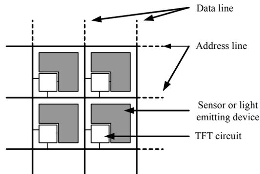
**Fig. 2.2 General schematic of an active matrix array.**
