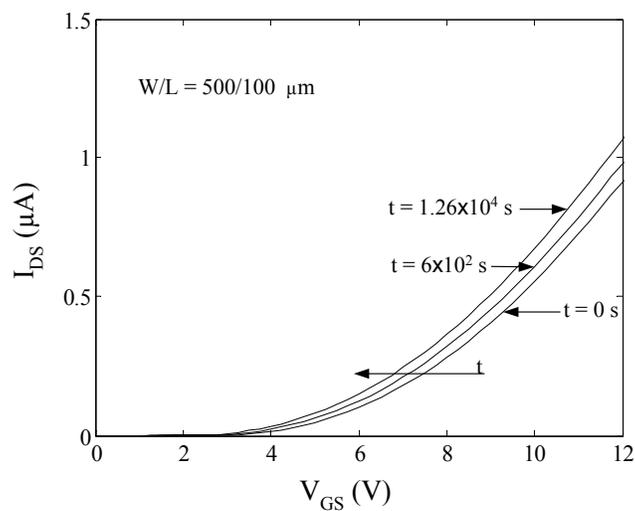
**Fig. 4.1 Transfer characteristics of a TFT at different times after removing the 20V bias stress (the aspect ratio of TFT is  $W/L = 500/100 \mu m$ ).**
