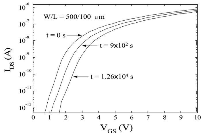
**Fig. 3.3 I-V characteristics of a TFT plotted on a semi-logarithmic scale after  $t = 0, 9 \times 10^2$ , and  $1.26 \times 10^4 \text{ s}$  of the application of a 20V gate bias stress ( $V_{DS} = 0 \text{ V}$  during the stress)**
