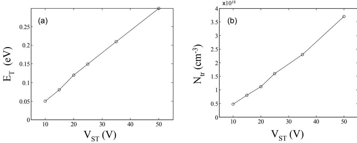
**Fig. 4.10 (a)  $E_T$  and (b)  $N_{tr}$  are extracted from the threshold voltage relaxation results after removing 3.5 hours of bias stress with different stress voltages.**
