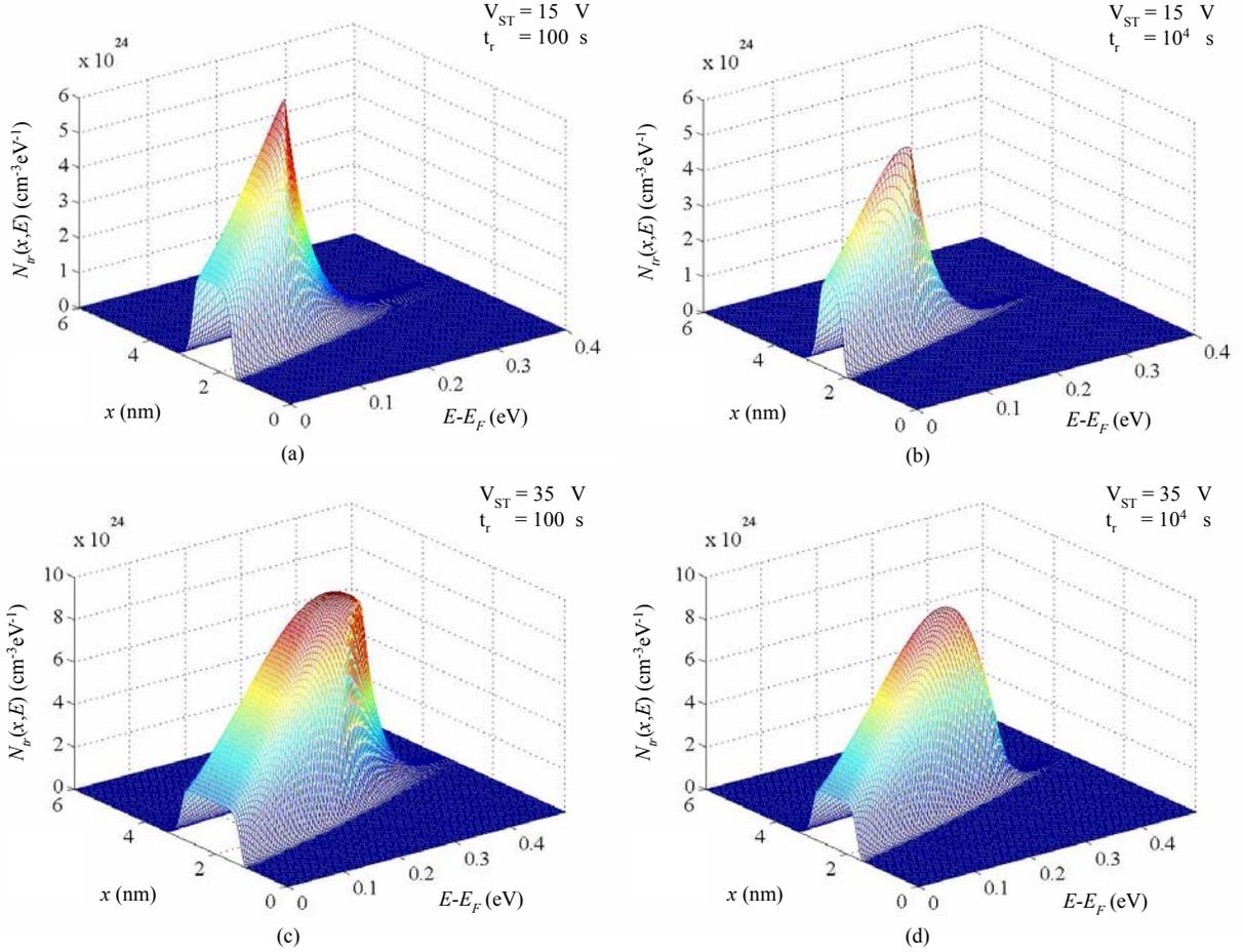
**Fig. 4.11 Concentration of filled traps as a function of the distance and energy after 100 and  $10^4$  seconds of removing (a), (b) a 15V bias stress and (c), (d) a 35V bias stress for 3.5 hours.**
