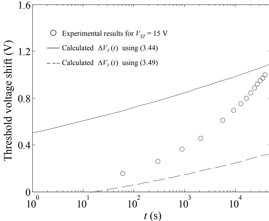
**Fig. 3.15** Calculated threshold voltage shift using (3.49) (dashed line) and (3.44) (solid line); the experimental results of  $\Delta V_T(t)$  due to a 15 V bias stress are also shown (open circles).
