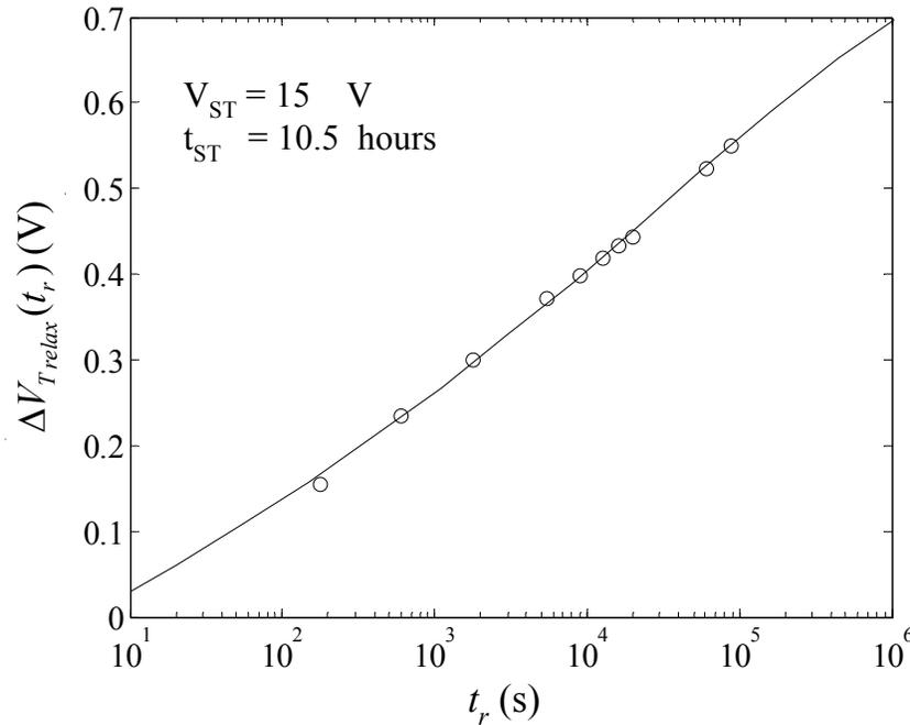
**Fig. 4.13** Threshold voltage relaxation calculated using (4.24) (solid line), and the experimental results (open circles) after 10.5 hours of bias stress with 15V.
