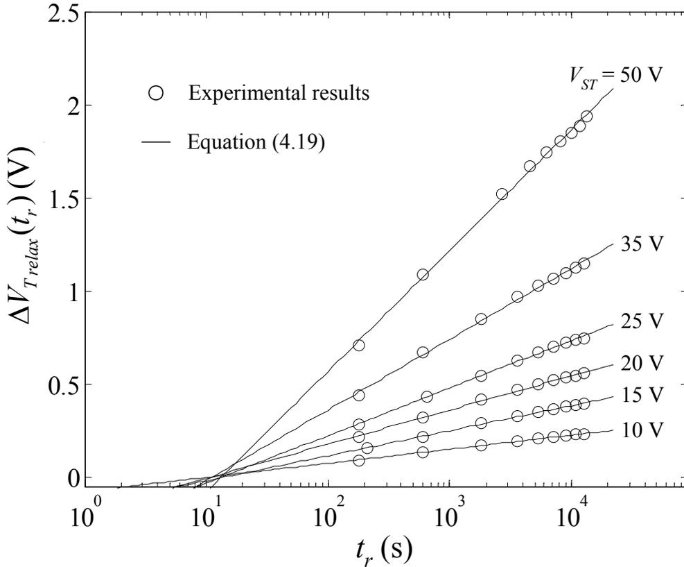
**Fig. 4.9** Solid lines are the result of the least-square fitting of (4.19) to the experimental threshold voltage relaxation after different bias stress tests for 3.5 hours (open circles).
