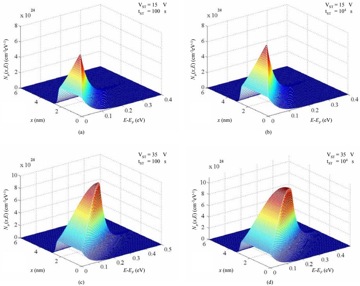
**Fig. 3.13** Concentration of trapped electrons in SiN as a function of the distance from a-Si:H interface and energy level of trap states after 100 and  $10^4$  s of 15 and 35V stresses.
