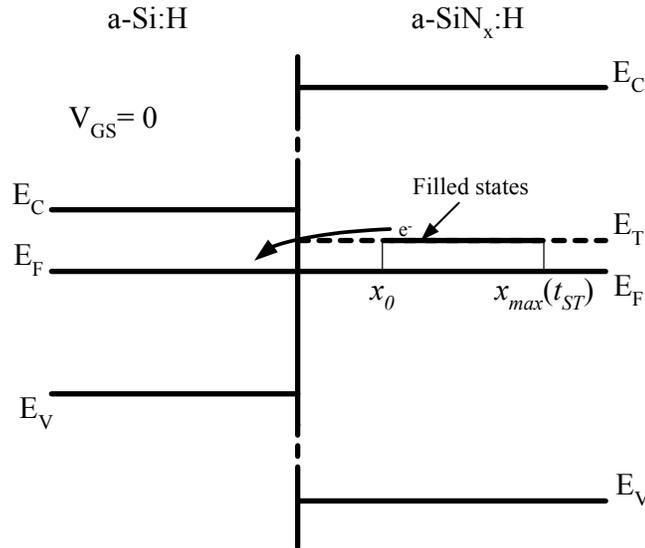
**Fig. 4.6 Energy-band diagram of the a-Si:H TFT near the gate dielectric interface after the removal of the bias stress for  $t = t_{ST}$ .**
