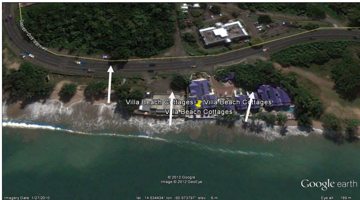
Figure 12: Villa Beach Cottages- Beach is Lost Even if Seawall Protects Pool Area and Property
