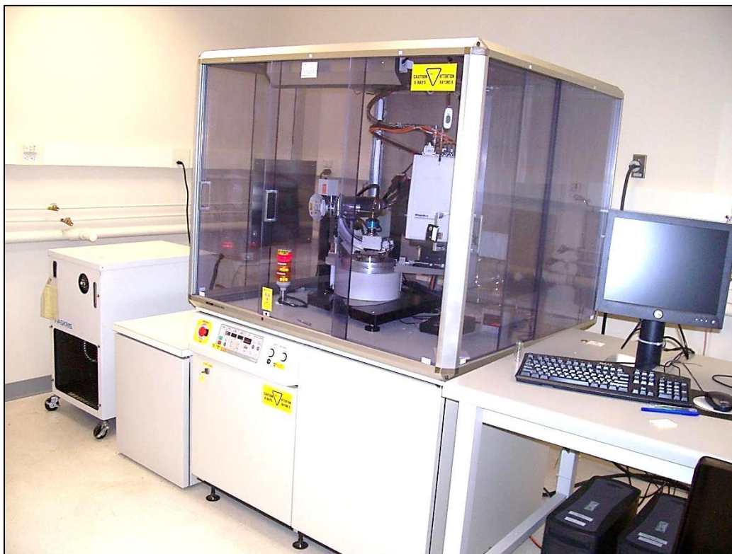
Figure 3-4 X-Ray Diffraction equipment for phase analysis of samples-From CAMJ lab 126
