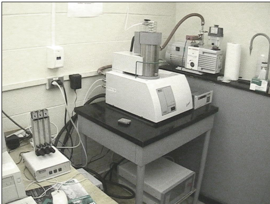
Figure 3-3 Netzsch STA machine used for thermal analysis-From the reference 125
