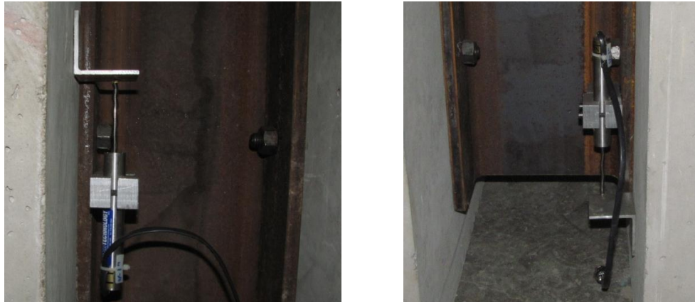
Figure 4-23: Top (Left) and Bottom (Right) Configuration of the Displacement Transducers
