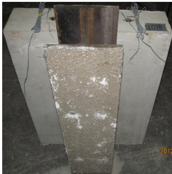
Figure 5-19: Friction Enhanced Steel Flange Surface after Testing – Specimen FE1 L-53
