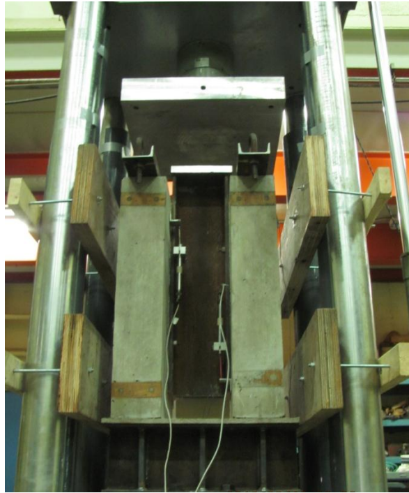
Figure 4-21: Typical Push Test Setup
