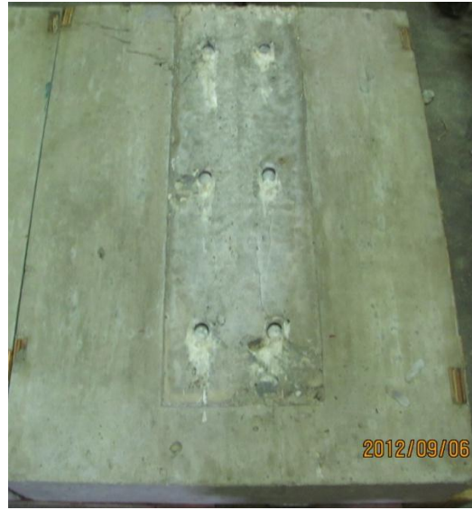
Figure 5-1: Shear Studs Fracture Failure (Left); Fractured Studs in Concrete Slab (Right)
