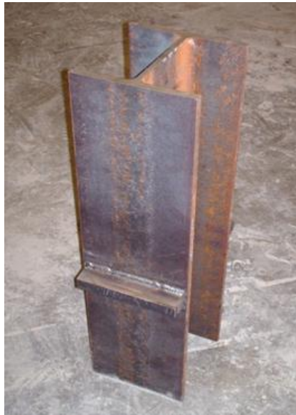
Figure 4-7: Shear Lug Specimen – Before Concrete Casting
