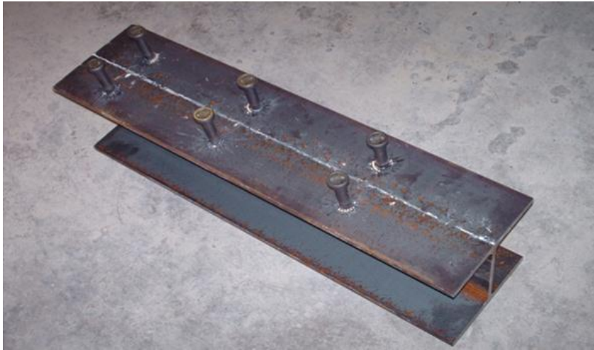
Figure 4-6: Shear Stud Specimen – Before Concrete Casting
