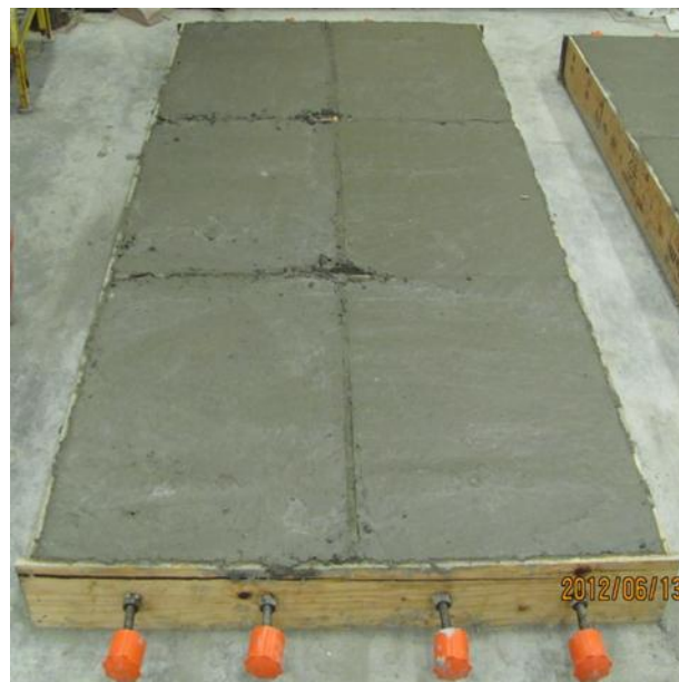
Figure 4-14: Concrete Slabs after Casting (Top and Bottom)
