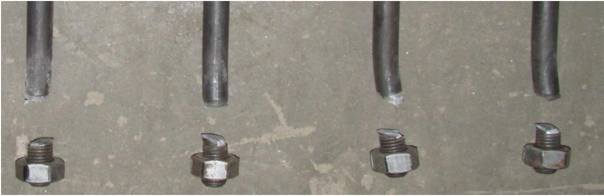
Figure 5-6: Close Up Shot of the Fractured Bolt Surface – Specimen P M-85
