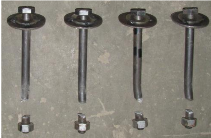
Figure 5-5: Fractured Bolts After Testing – Specimen P M-85
