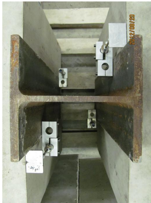
Figure 4-22: Placement of Four Displacement Transducers
