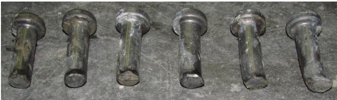
Figure 5-2: Fractured Shear Studs After Testing
