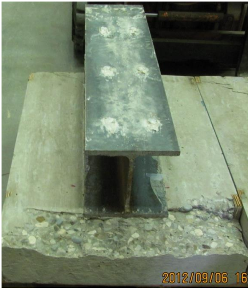
Figure 5-1: Shear Studs Fracture Failure (Left); Fractured Studs in Concrete Slab (Right)
