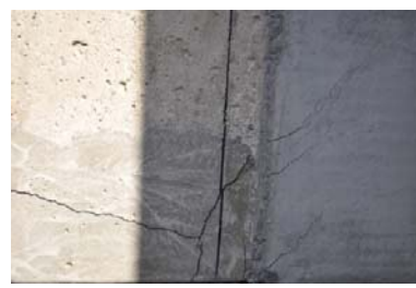
Critical crack location (back view)
