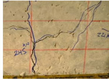
Dominated flexural crack
