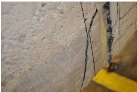
Critical shear-bond crack (front view)
