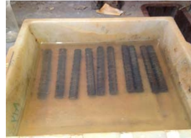
(b) Soaking the steel sections in the solution
