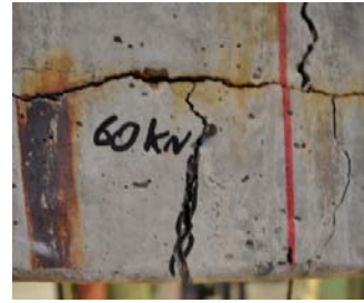
Dominated flexural crack
