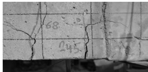
Dominated flexural crack
