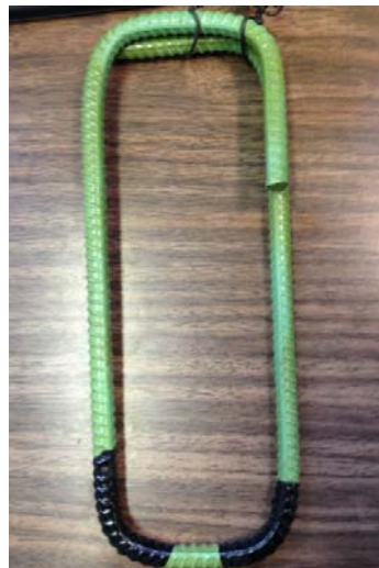
Figure 3.4: Protection and insulation of stirrups
