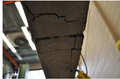
Bottom view for the failure zone
