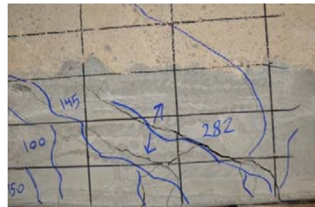
Critical inclined shear-bond Crack
