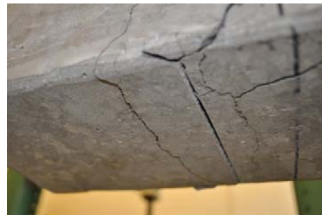
Critical shear-bond Crack (back view)
