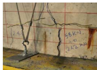
Dominated flexural crack
