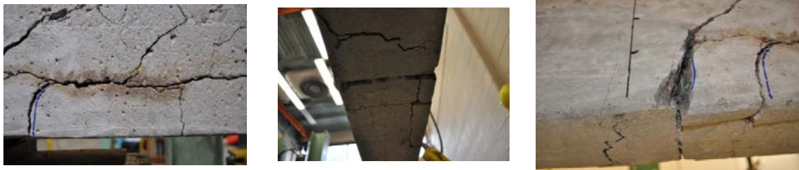
(a) Splitting bond failure
