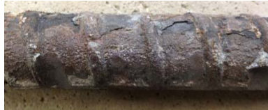
(b) Exposure time 30 days (2.5 % mass loss)
