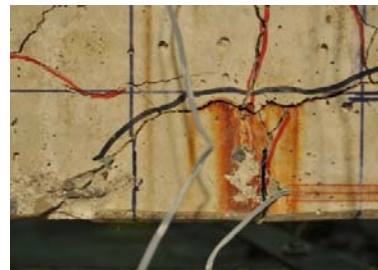
Dominated flexural crack
