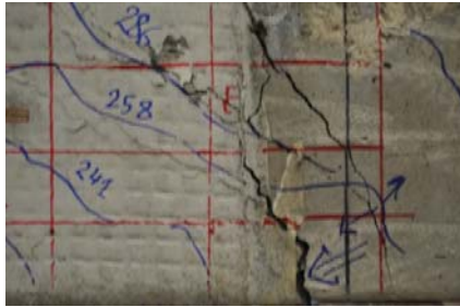
Critical shear-bond crack (front view)
