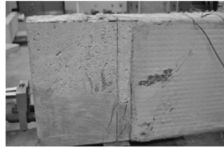
Critical crack location (back view)
