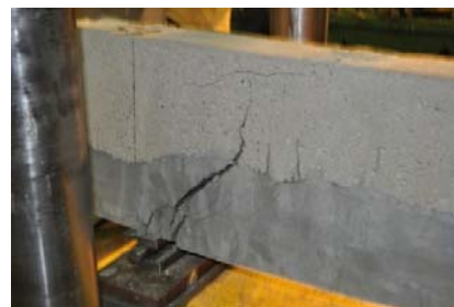
Critical inclined shear-bond Crack
