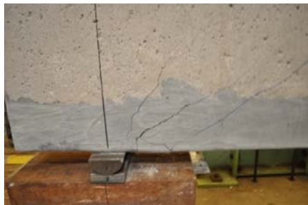
Propagation of Splitting crack
