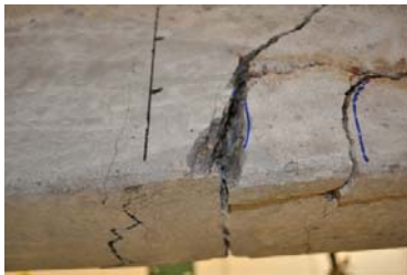
Back view for the anchorage failure
