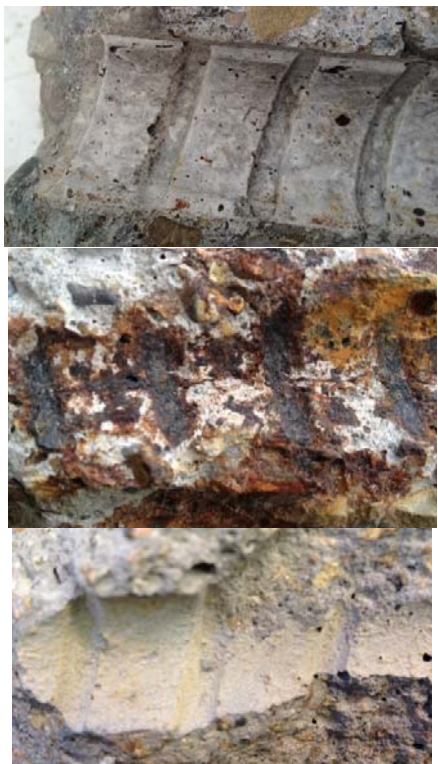
Figure 4.15: Concrete below the steel in the test specimens
