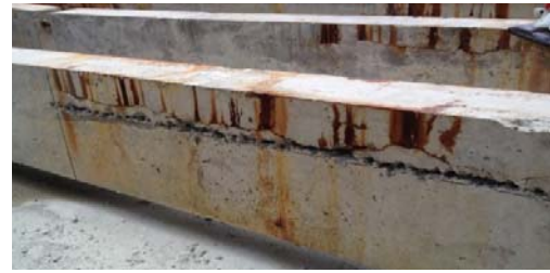
(b) Drilled holes along the deteriorated zone
