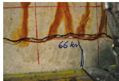
Dominated flexural crack
