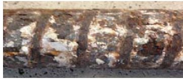
(c) Exposure time 60 days (5 % mass loss)
