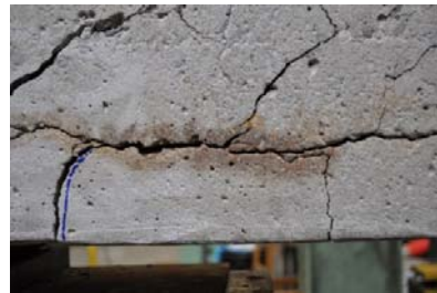
Splitting induced cracks
