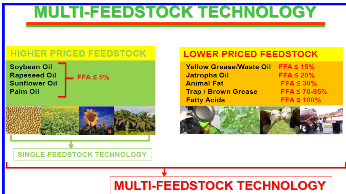
Figure 5.1 Schematic presentation of multi-feedstock biodiesel technology to produce biodiesel from 1 st and 2 nd generation feedstocks.
