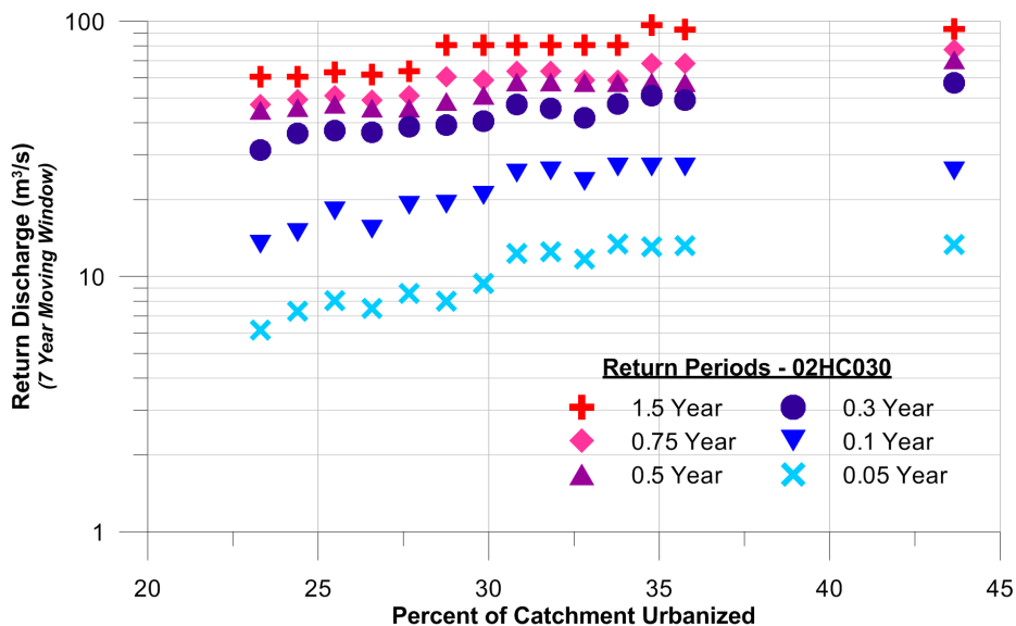
Figure 4.28: Change in Various High Frequency Return Discharges at Etobicoke Creek below QEW comparing with Urbanization (02HC030)
