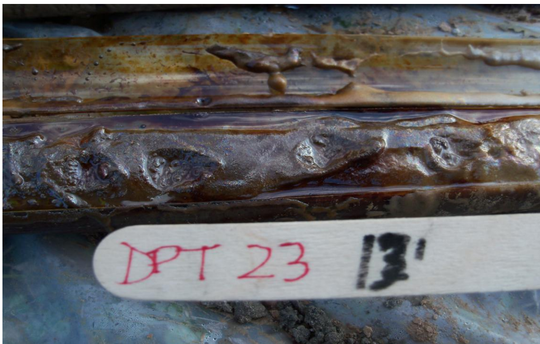
Figure G.4. NAPL saturated pores in DPT-23 at 13 ft bgs.
