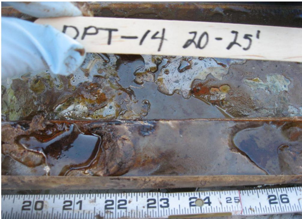
Figure G.3. NAPL saturated pores in DPT-14 at 20-25 ft bgs.
