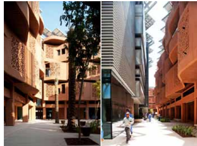
Figure 3.29 The buildings are configured to create narrow, colonnaded urban spaces that are in shade for much of the day
