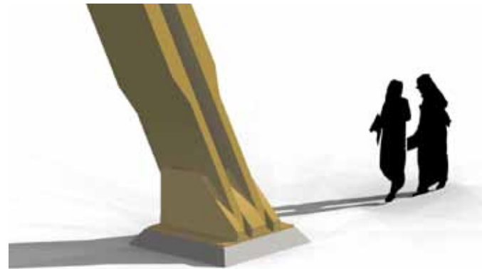
Figure 4.58 Column base connection (fixed)
