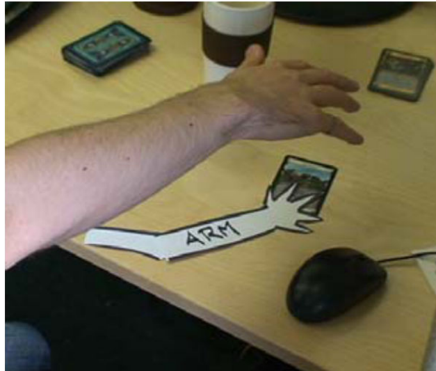
Figure 34: Mocked-up design concept of an Adapted Pick and Drop arm shadow. The arm representation follows the movement of the user's arm until the hand's contents are dropped
