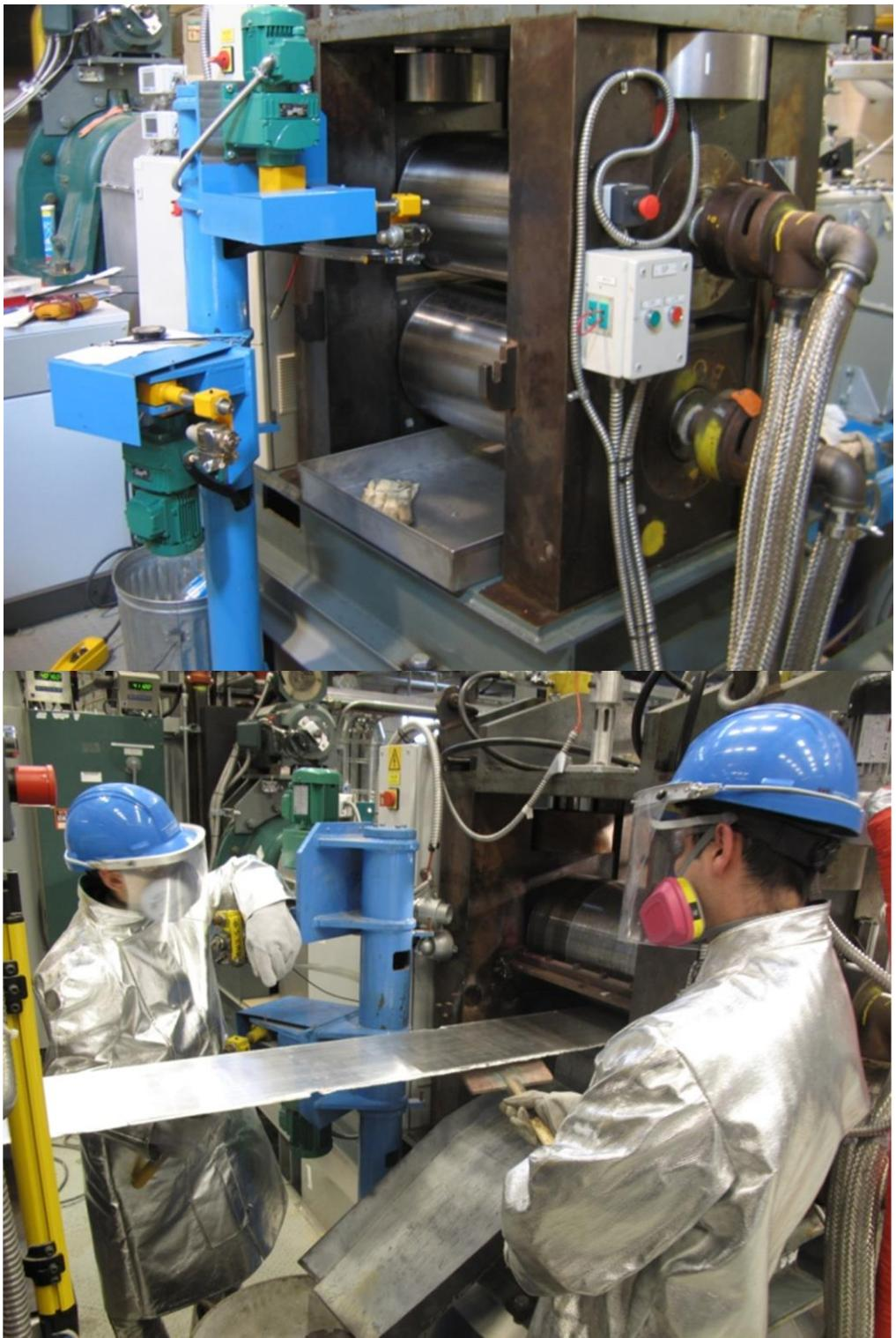
Figure 4-1- Twin roll caster at CanmetMATERIALS used for magnesium alloys [19].
