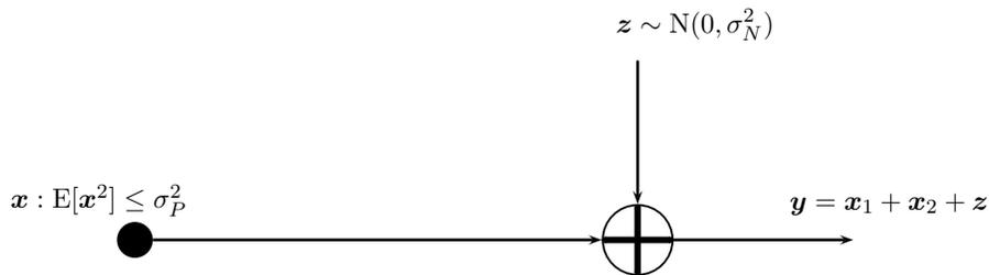
Figure 1.1: A point-to-point additive white Gaussian noise channel with average power constraint at the transmitter
