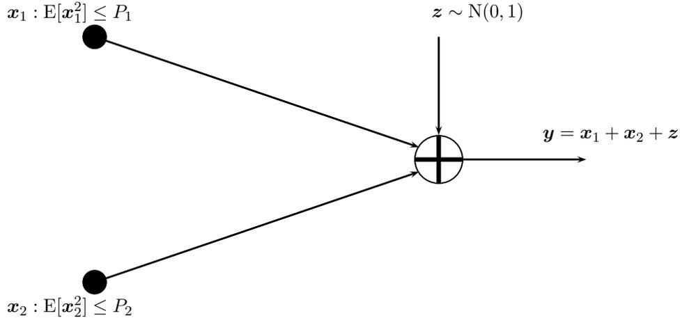
Figure 3.3: A two-user Gaussian multiple access channel with average power constraints
