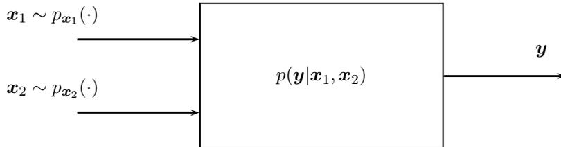
Figure 3.1: A two-user multiple access channel
