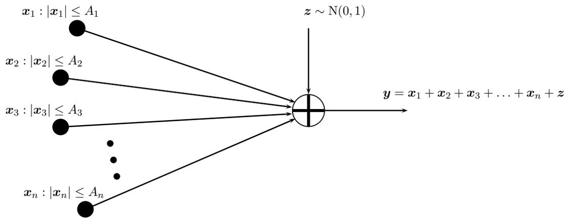
Figure 3.5: n-user Gaussian multiple access channel with peak constraints
