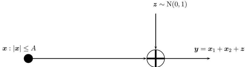
Figure 2.1: A point-to-point additive white Gaussian noise channel with peak power constraint at the transmitter
