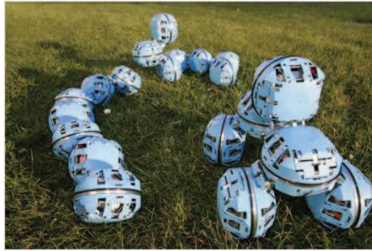
Figure 1-1: Atron, a Hybrid and Lattice MRR [11]
