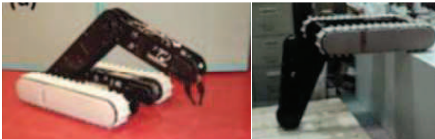
Figure 1-11: HMR, Hybrid Approach to Mobility Enhancement [10]
