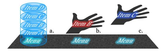
Figure 2.3. Spatial menu used in LightSpace installation: a. virtual menu items are placed at different heights, b. and c. when a hand is held at certain heights the corresponding items are projected onto it
