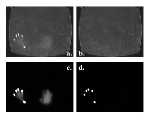
Figure 4.4. Image processing in the tracker: a. original image, b. extracted background, c. hover layer, d. touch layer
