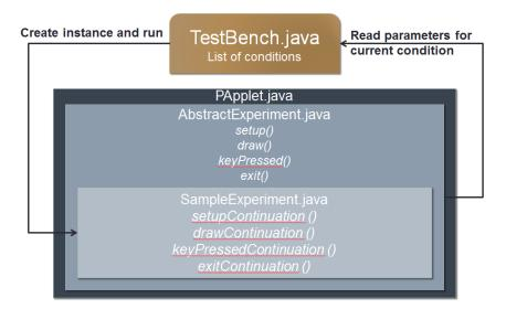
Then, TestBech class creates an instance of an experiment class, which extends AbstractExperiment class and/or PApplet class and runs it. The experiment class implements abstract methods of AbstractExperiment class to extend its functionality.
