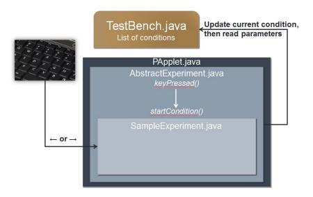
AbstractExperiment class captures key press events and when left and right arrow keys are pressed, it calls functions *nextCondition()* and *previousCondition()* of TestBench class to change the current condition and then reads the new set of parameters from TestBench.
