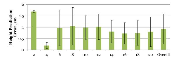
Figure 4.7. Mean error of prediction at each height (from 2 to 20 cm) and overall (error bars represent standard deviation)
