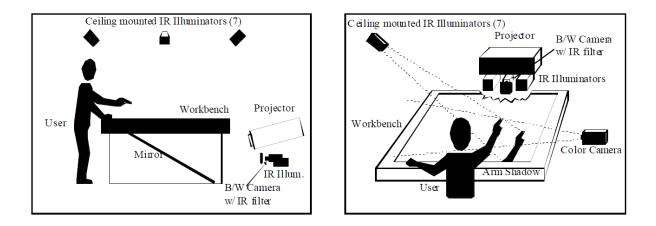
Figure 2.2. Perceptive Workbench, light and camera positions 5
