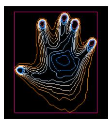
Figure 4.5. Visualization of the height data produces by the Slices method: orange outlines represent the dimmest parts of the image, blue outlines represent brighter parts and red outlines represent touch regions
