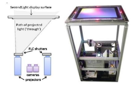
Figure 2.5. The layout of the main components of SecondLight 7
