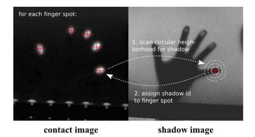
Figure 2.4. A contact image and a shadow image used in Shadow Tracking system <sup>6</sup>
