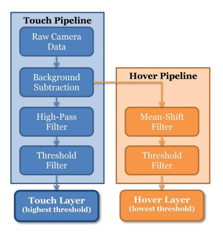
Figure 4.3. Touch and hover pipelines used in the tracker
