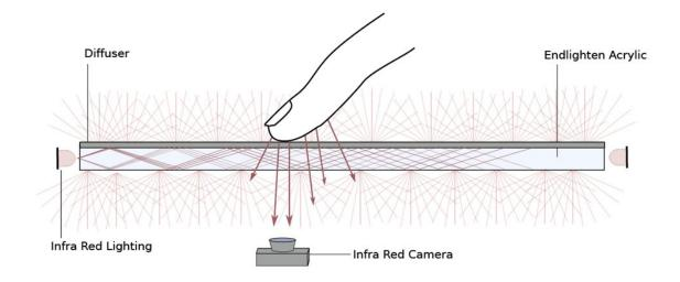
Figure 4.1. The main components of a DSI setup <sup>11</sup>
