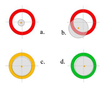
Figure 5.3. The targets (circular rings) and cursor used in experiment 2. Targets first appears red (a. & b.), turns yellow when acquired (c.) and green upon selection (d.). The radius of the cursor is determined by the height of the participant's hand above the table.
