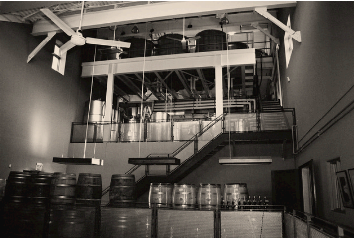
Figure 52: Tawse' Six-Level Gravity-Fed Processing System (Nowpublic.com, 2008)
