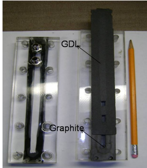
Figure 3.5: Graphite channel covered with hydrophobic GDL for pressure measurements.
