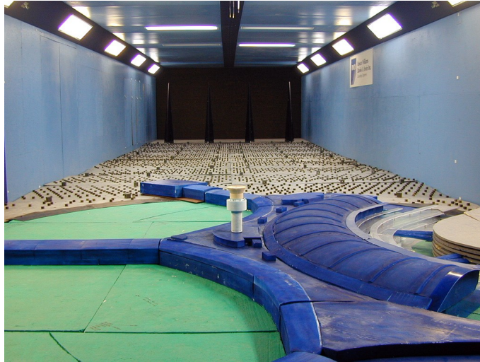
Figure 7.14: High frequency base balance wind tunnel study model of Pearson International Airport Apron Tower (Courtesy Rowan Williams Davies and Irwin Inc.)
