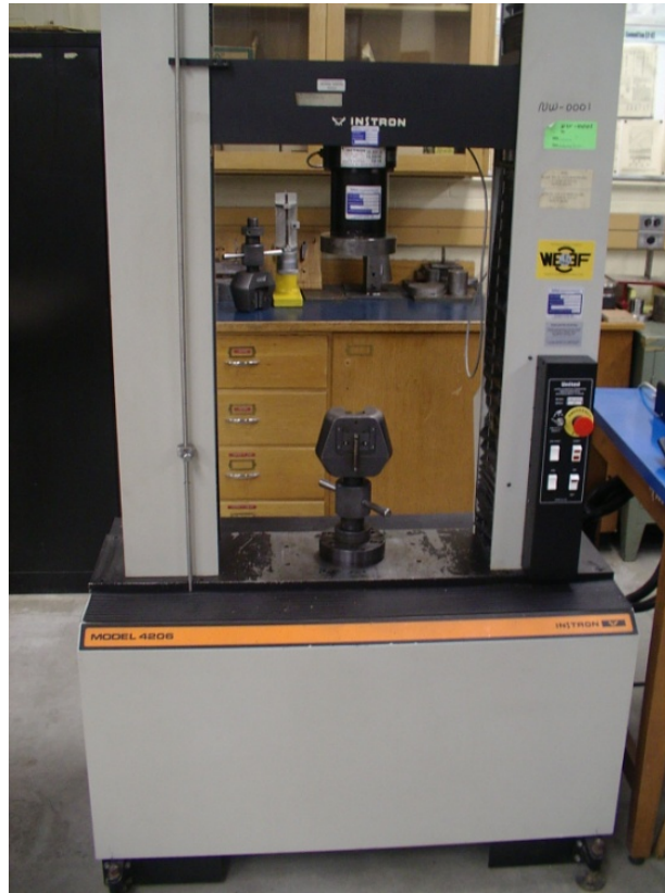
Figure 48: Instron universal testing machine model 4206
