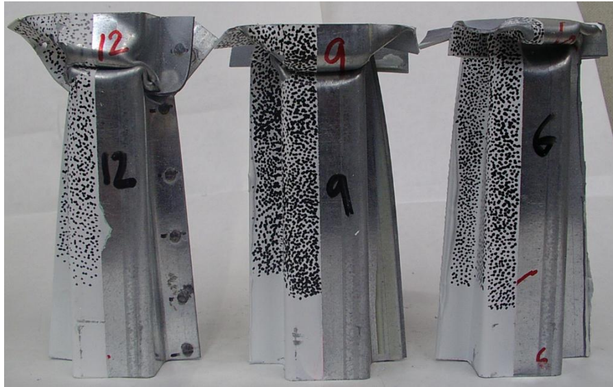
Figure 68: Dynamic impact deformed hats. Spot welded (left), bonded DP-460NS (center), and bonded EC-2214 (right)
