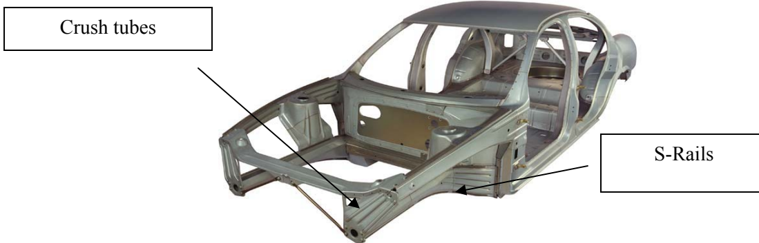
Figure 2: Energy absorption components in automotive structures [38]
