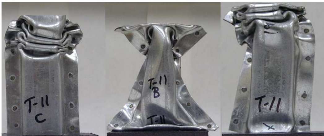
Figure 53: Deformed welded hat sections during QS testing
