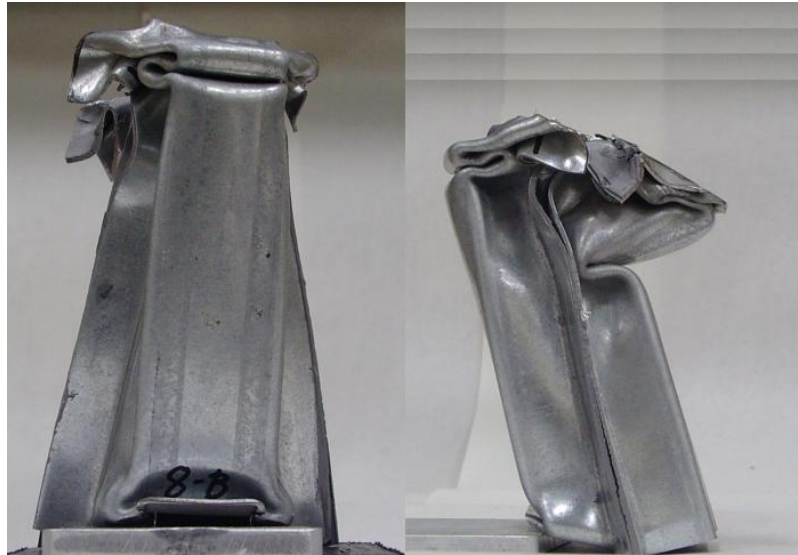
Figure 56: Specimen-8B; transition from crushing to global bending during test
