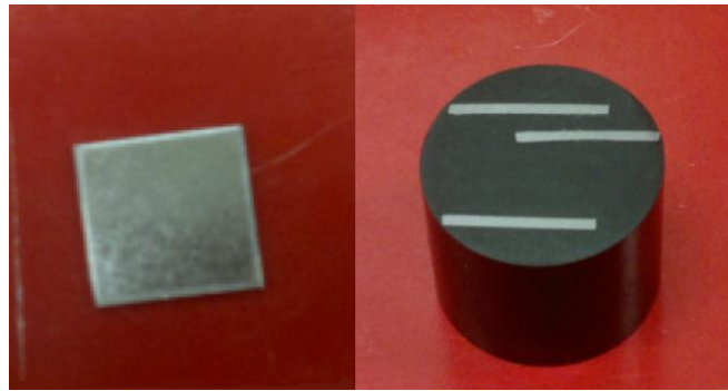
Figure 45: Micro-hardness test samples. Cut material (left), mounted material on Bakelite (right)
