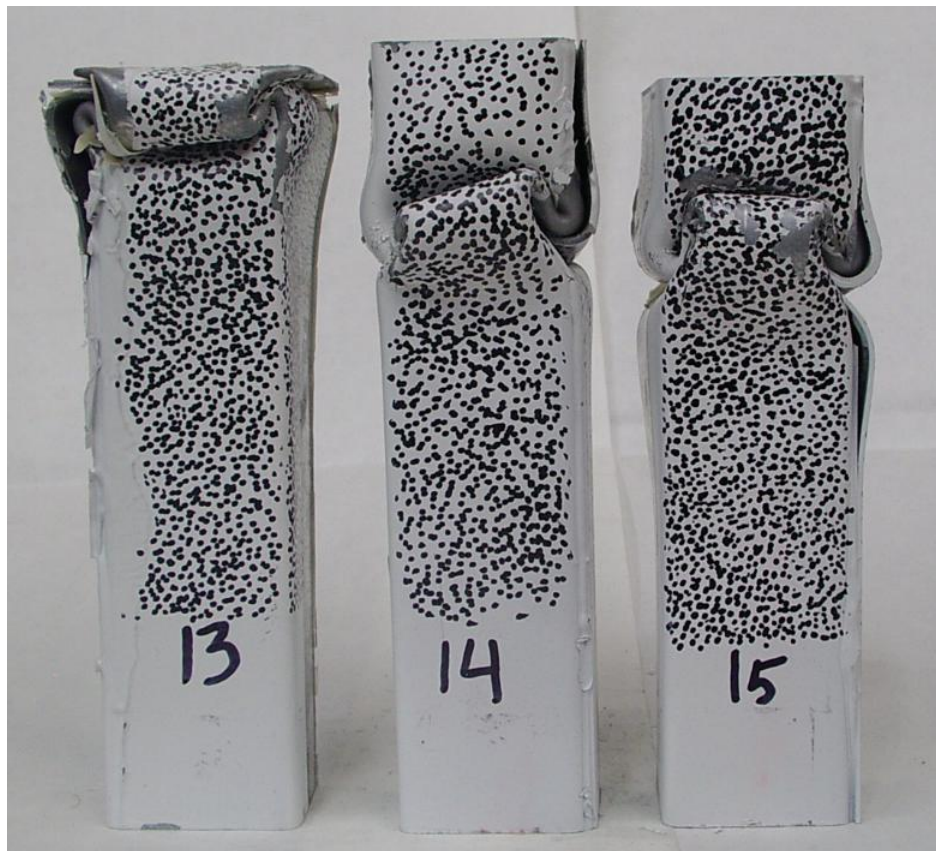
Figure 74: Dynamic impact, channels bonded with DP-460NS
