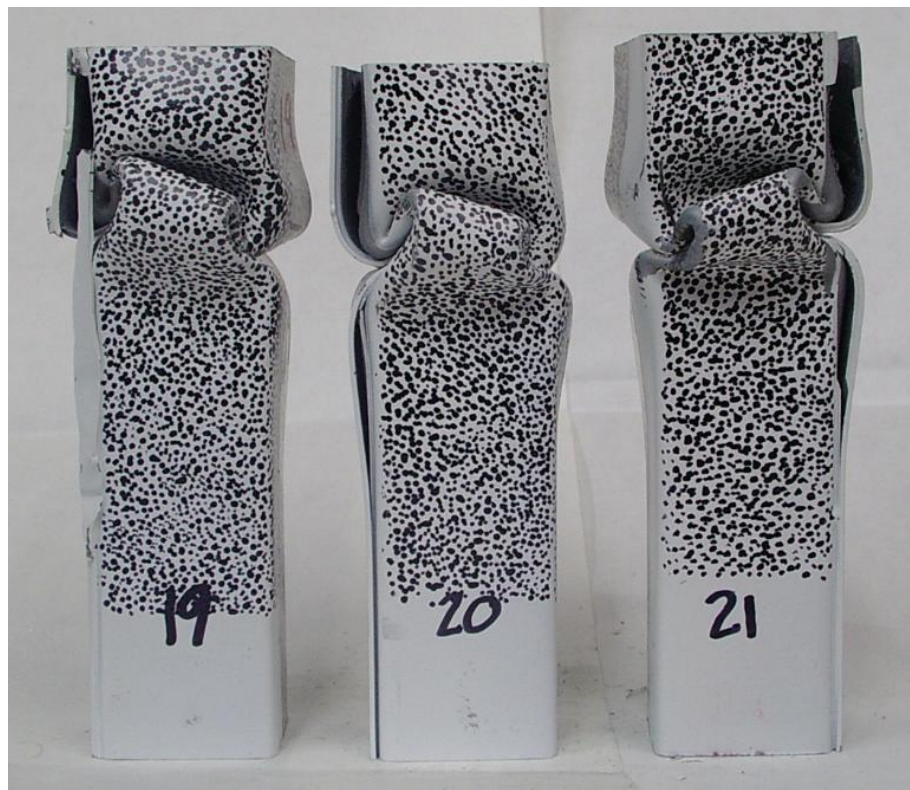
Figure 76: Dynamic impact, channels bonded with EC-2214
