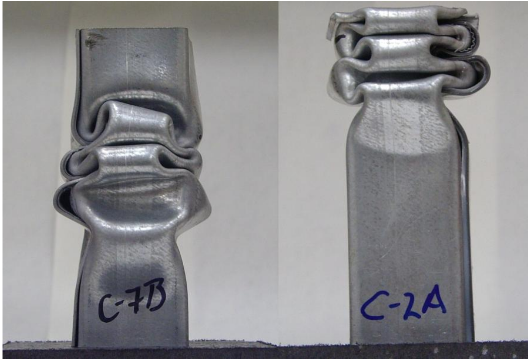
Figure 58: Deformed channel sections during QS testing. Bonded EC-2214 (right), bonded DP-460NS (left)
