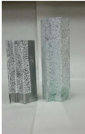
Figure A 5: Paint job for DIC system
