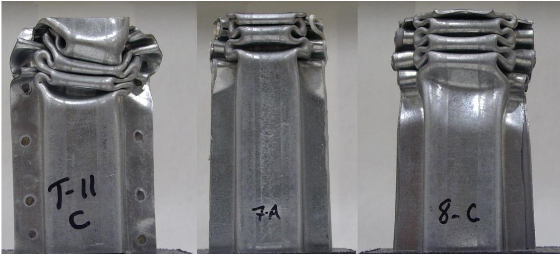
Figure 52: Deformed hat sections during QS testing. Welded (left), bonded DP-460NS (center), bonded EC-2214 (right)
