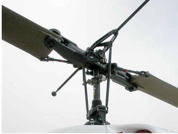
Figure 2.2: Stabilizer Bar on Bell 212/HH-1N rotor head. Photo: Alan K. Radecki (CC BY-SA 3.0)
