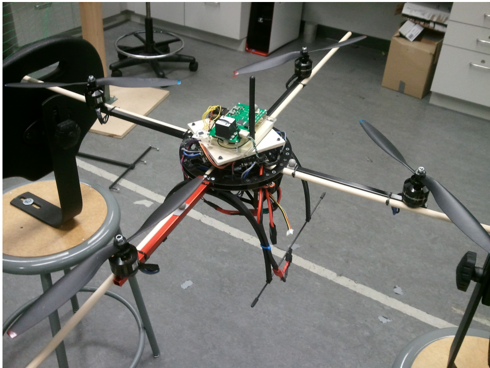
Figure 4.9: Quadrotor in a constrained testbench
