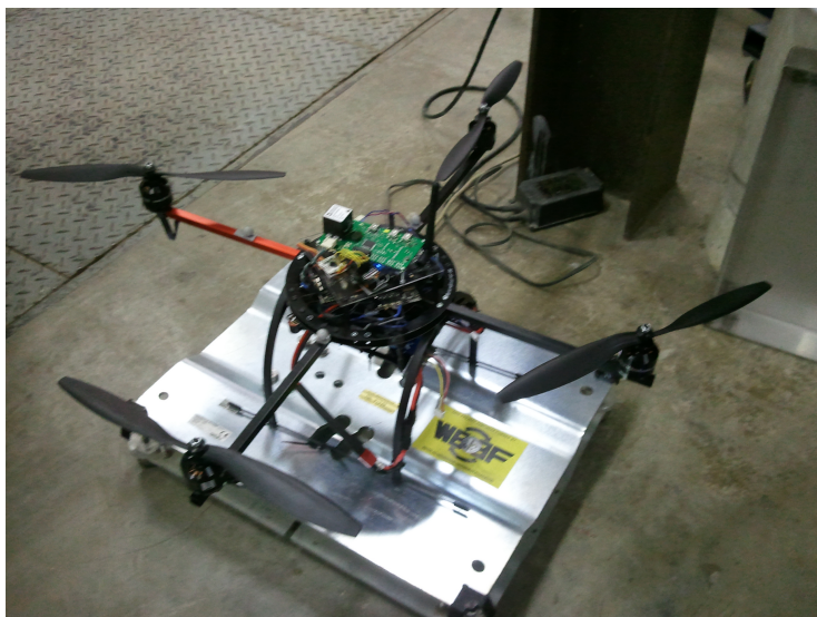
Figure 4.6: Quadrotor platform mounted on a Scale for thrust study
