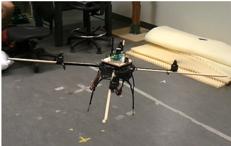
Figure 4.8: UWMAV Autopilot mid flight on the Mikrokopter
