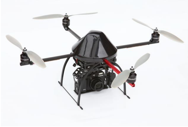
(a) Stock Mikrokopter Quadro XL being using for Aerial Photography
