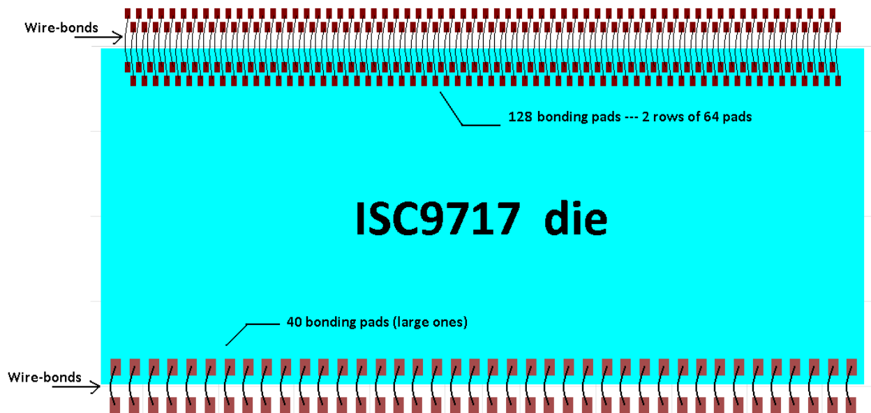
Figure 2.3 – Can the Indigo Silicon die be wire-bonded to PCB like this?
