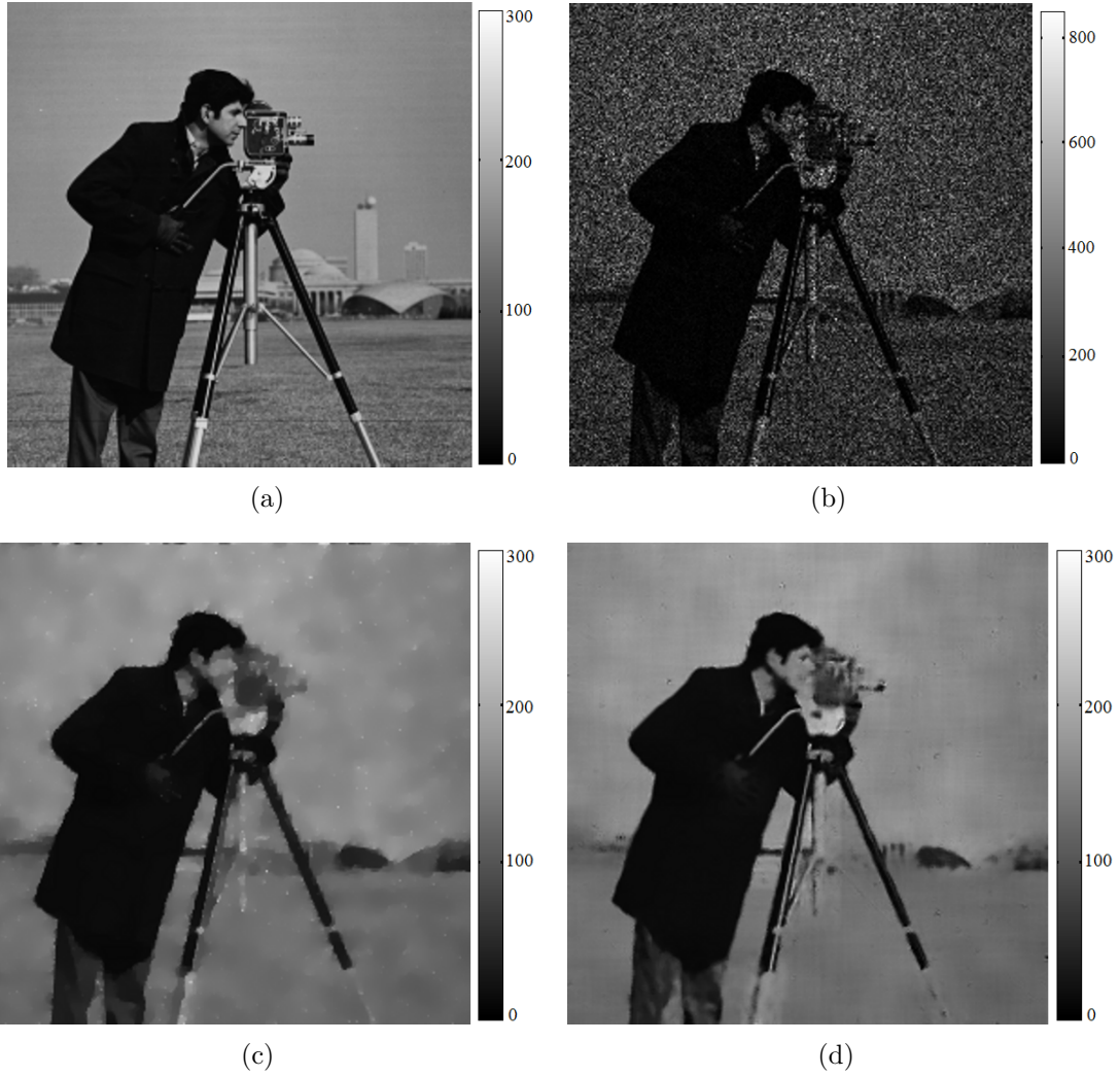
Figure 6.1: (a) Original image; (b) Noisy image (SNR = 3.1018 dB, SSIM = 0.2191); (c) Reconstruction using the method of [30] (SNR = 17.1836 dB, SSIM = 0.7134), and (d) Reconstruction using NLM filtering with the proposed C^S (SNR = 18.1878 dB, SSIM = 0.7176).
