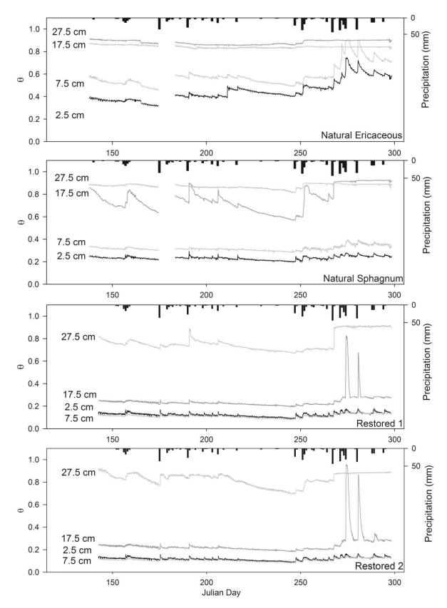
Figure 3-1 Time-series  $\theta$  from in-situ measurements at 4 sites (2 RES and 2 NAT) from DOY 145-290. RES (bottom) show limited variability between the 2.5 and 7.5 cm probes and overall low  $\theta$  above the cutover peat/*Sphagnum* interface. NAT probes were placed under a pure *Sphagnum* hummock and an ericaceous covered hummock and show large differences in the  $\theta$  of the upper 3 probes.
