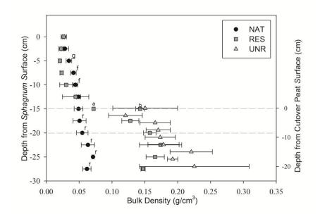
Figure 3-2 Bulk density by samples depth centered at 2.5 cm for all three sites. Between the dashed grey lines represent the interface region between the cutover peat and *Sphagnum* moss at RES. The 15 cm RES samples were split into two groups of 2 (denoted by <sup>a</sup> or <sup>b</sup>) based the dominant material type (*Sphagnum* or cutover peat). n=4 per site
