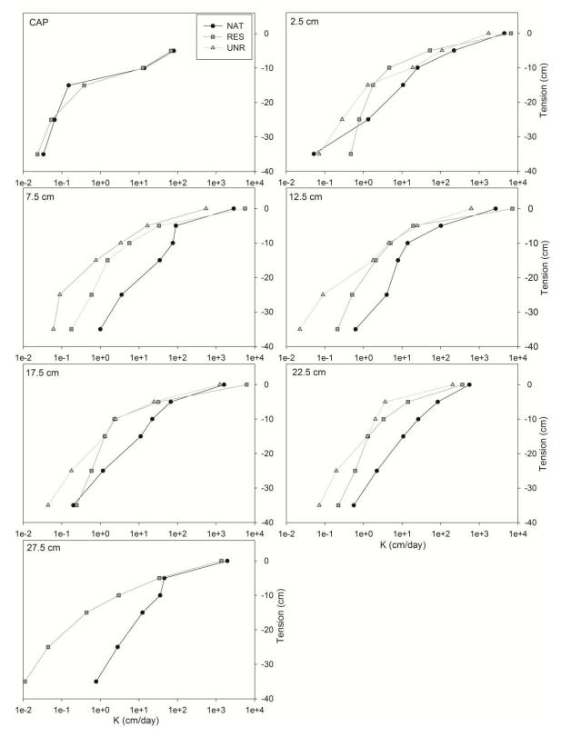
Figure 3-6 Hydraulic conductivity and  $\psi$  from the monolith parameterization for each sample depth. RES 22.5 and 27.5 cm are within the cutover peat and the 17.5 cm sample is within the transition zone between cutover peat and *Sphagnum* moss. The hysteretic curves were removed for clarity but follow the same general trends as the soil water retention hysteretic curves.
