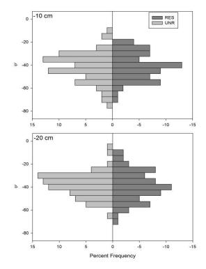
Figure 2-6 Histograms of soil water pressures at 10 and 20 cm below the cutover peat surface (~30 and 40 cm below the regenerated *Sphagnum* surface). RES and UNR had similar average soil water pressures at both depths. The cutover peat/*Sphagnum* interface was at ~ 20 cm below the surface.
