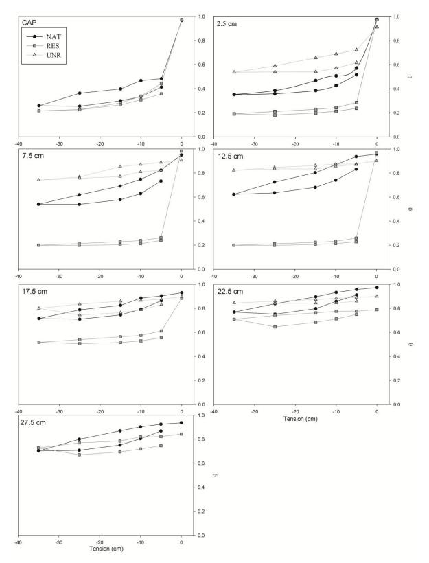
Figure 3-5 Soil water retention and hysteresis curves from the monolith parameterization for each sample depth. RES 22.5 and 27.5 cm are within the cutover peat and the 17.5 cm sample is within the transition zone between cutover peat and *Sphagnum* moss.
