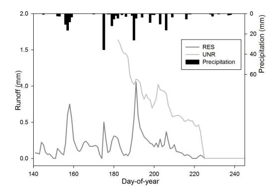
Figure 2-2 Runoff depth (mm) over time from RES and UNR from D 140 – 245. UNR started on D 182 due to the site outflow being blocked.
