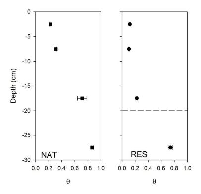
Figure 2-3 Average volumetric soil moisture contents of the *Sphagnum* and cutover peat at RES and NAT. Measurements centred at 2.5, 7.5, 17.5, and 27.5 cm below the *Sphagnum* surface. The dashed grey line represents the approximate interface between the regenerated *Sphagnum* moss and the cutover peat. Error bars indicate 1 standard deviation. All NAT measurements are significantly different than RES at p= 0.001.
