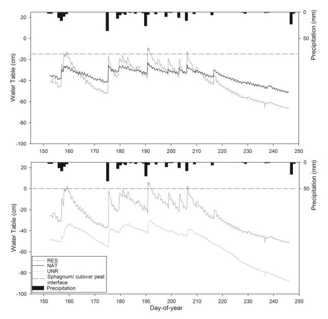
Figure 2-4 Water tables over time (D 145-245) generated from the continuous water table data. RES and NAT's datum are referenced to the top of the Sphagnum moss. RES and UNR's datum are referenced to the top of the cutover peat, ~15 cm below the regenerated *Sphagnum* moss at RES.
