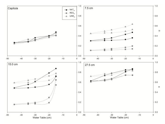
Figure 3-3 Average  $\theta$  results from the monolith experiments for each probe (n=2) and the capitula peatboard (n=9). The capitula, 7.5 and 15.0 cm measurements are within the *Sphagnum* at RES and the 27.5 cm measurements is within the cutover peat at RES.
