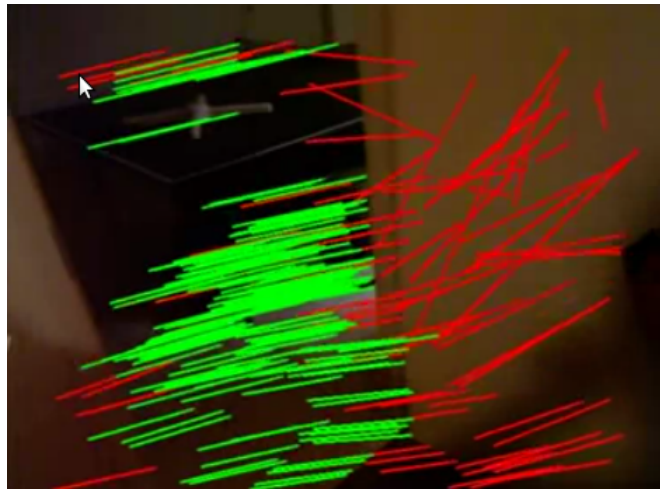
Figure 3.3: RANSAC based visual odometry
