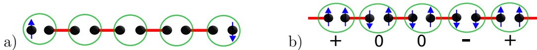
Figure 3.1: A cartoon diagram of the spin-1 Haldane phase. The red bonds represent spin-1/2 singlet states. The green circles are effective spin-1 states formed by the neighbouring halves of two singlet bonds. Fig. a) shows that on a chain with open boundary conditions one needs to include free spin-1/2's on the edges. Fig. b) shows a possible state where each site has S_z either 1, 0 or -1.
