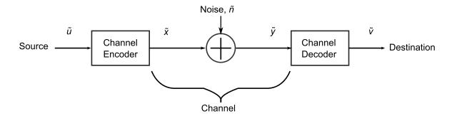
Figure 2.3: Basic Communication System. Channel modulator and demodulator are not shown in the picture.
