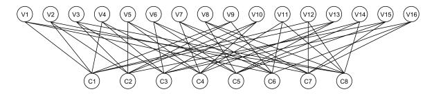
**Figure 2.2:** Tanner graph representation of the H matrix in Figure 2.1. Variable nodes are shown on top, and check nodes at the bottom
