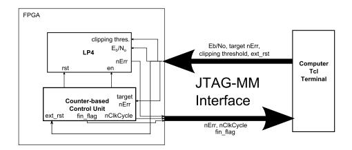
Figure 3.9: Interaction between LP4 core on the FPGA and computer Tcl terminal
