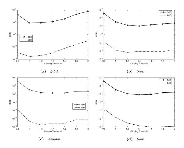
Figure 6.4: Information BER at  $E_b/N_0$  of 2 dB to 8 dB for configurations with 6 decoder cores on DE4 with various bit-widths for LLRs at a 75MHz clock with coded throughput of 2.4 Gbit/s for the  $T_s = 192$ ,  $\rho = 16$ , rate-1/2 (3,6) PN-LDPC-CC code using clipping thresholds from 0.8 to 2 during quantization. The 5-dB curves are based on a target number of errors of 100, while the 6-dB curves are based on a target number of 5.
