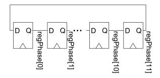
Figure 3.3: One-hot encoding of the phase signal for the  $T_s = 192$ ,  $\rho = 16$ , rate-1/2 (3,6) PN-LDPC-CC, group period  $T'_s = 12$ . [1]
