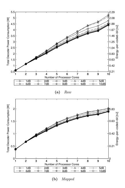
Figure 5.3: Average measured decoder power and energy-per-coded-bit at various  $E_b/N_0$  for various numbers of decoder cores on DE4 with 4-bit LLRs at a 75MHz clock with coded throughput of 2.4 Gbit/s for the  $T_s = 192$ ,  $\rho = 16$ , rate-1/2 (3,6) PN-LDPC-CC code based on three sets of measurements for each data point.
