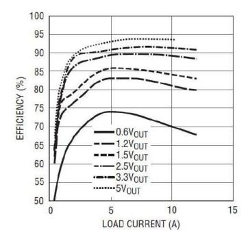
**Figure 4.3:** Efficiency versus Load Current with 12-V Input for LTM4601 Regulator. (Taken from the LTM4601 data sheet [2])
