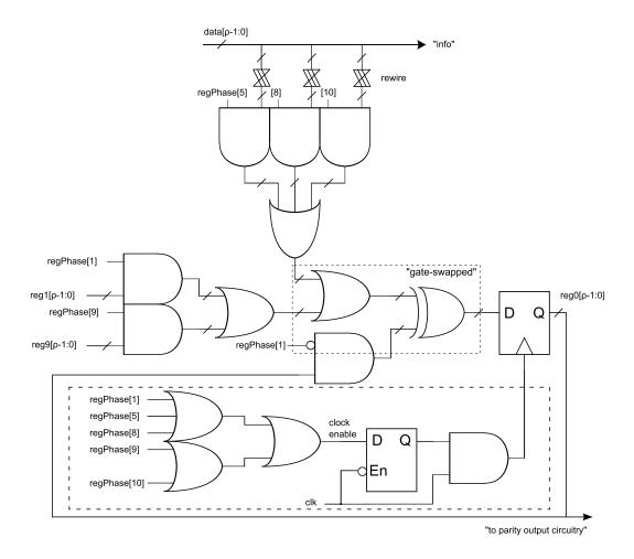
Figure 3.5: A single encoder node from the implemented architecture in this thesis for the  $T_s = 192, \ \rho = 16, \ rate-1/2 \ (3,6) \ PN-LDPC-CC. \ [1]$
