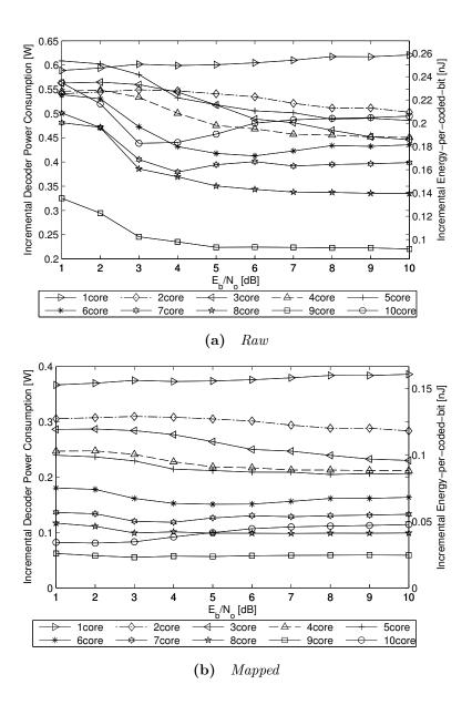
Figure 5.4: Incremental measured decoder power and energy-per-coded-bit for every dB of increase in  $E_b/N_0$  for various numbers of decoder cores on DE4 with 4-bit LLRs at a 75MHz clock with coded throughput of 2.4 Gbit/s for the  $T_s = 192$ ,  $\rho = 16$ , rate-1/2 (3,6) PN-LDPC-CC code.
