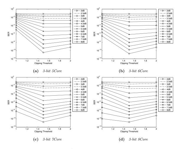
Figure 6.1: Information BER at  $E_b/N_0$  of 2 dB to 8 dB for configurations with 5 to 8 decoder cores on DE4 with 3-bit LLRs at a 75MHz clock with coded throughput of 2.4 Gbit/s for the  $T_s = 192, \rho = 16, rate-1/2$  (3,6) PN-LDPC-CC code using clipping thresholds from 1 to 2 during quantization.
