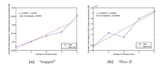
**Figure 4.1:** Decoder power obtained on configurations of 1 to 5 cores with Nios II unit incorporated using board power measurement method with mapping step and Nios II measurement unit
