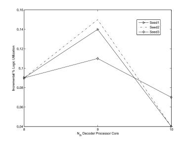
**Figure 5.7:** Incremental logic utilization for various configurations with 8, 9, 10 decoder processor cores
