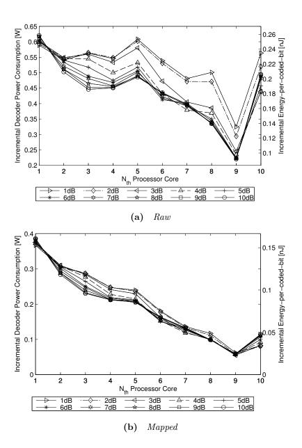
Figure 5.5: Incremental measured decoder power and energy-per-coded-bit for each additional core at various  $E_b/N_0$  on DE4 with 4-bit LLRs at a 75MHz clock with coded throughput of 2.4 Gbit/s for the  $T_s = 192$ ,  $\rho = 16$ , rate-1/2 (3,6) PN-LDPC-CC code.
