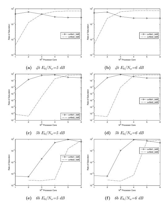
**Figure 6.3:** Rate of Saturation Events for "6Core" decoder with constant 4-bit, 5-bit, 6-bit LLRs at  $E_b/N_0$  of 5, 6 dB
