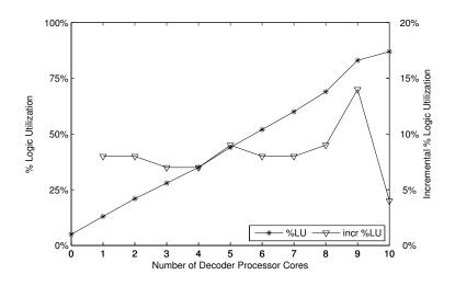
**Figure 5.6:** Logic utilization and incremental logic utilization for various configurations with different numbers of decoder processor cores
