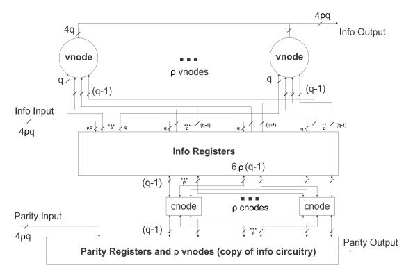
Figure 3.6: A single decoder processor. [1]
