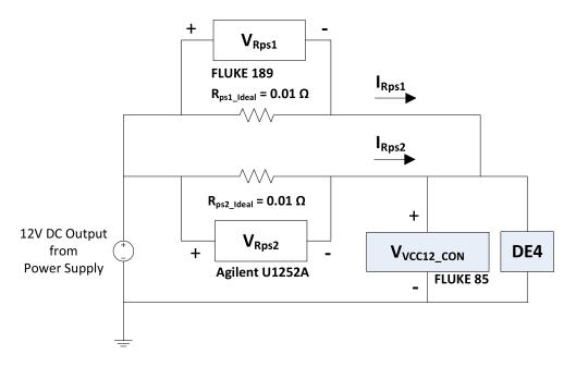
Figure 4.2: Power Measurement Set-up
