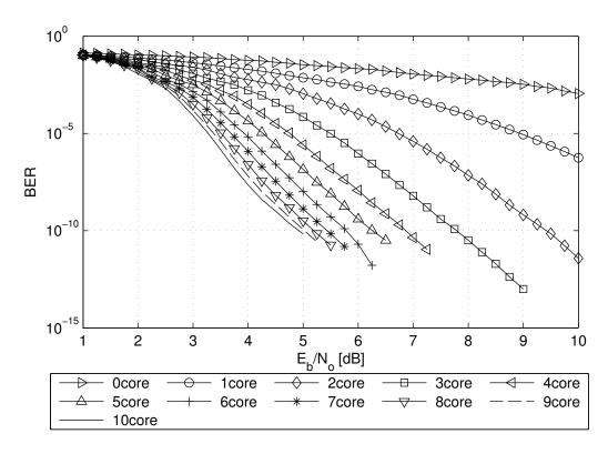
Figure 5.1: BER for various numbers of decoder cores for the  $T_s = 192$ ,  $\rho = 16$  rate-1/2 (3, 6) PN-LDPC-CC code with 4-bit LLRs at various  $E_b/N_0$  obtained from measurements on DE4 based a target number of errors of 1000 based on a BPSK-based AWGN channel.
