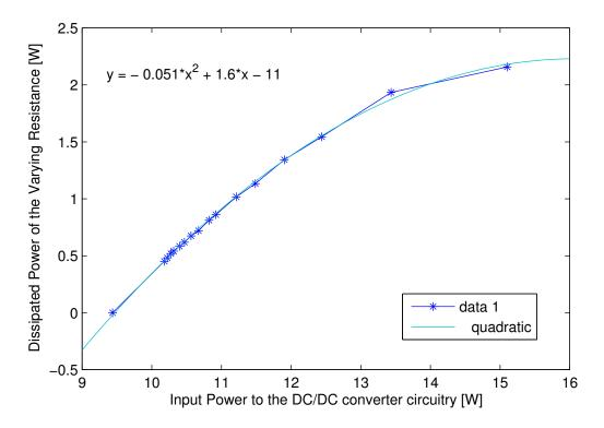
**Figure 4.5:** Input and output power measured for the DC/DC converter circuitry on the Altera DE4 using the setup denoted in Figure 4.4
