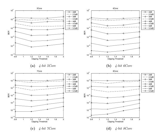
Figure 6.2: Information BER at  $E_b/N_0$  of 2 dB to 5.5 dB for configurations with 5 to 8 decoder cores on DE4 with 4-bit LLRs at a 75MHz clock with coded throughput of 2.4 Gbit/s for the  $T_s = 192, \rho = 16, rate-1/2$  (3,6) PN-LDPC-CC code using clipping thresholds from 0.8 to 2 during quantization.
