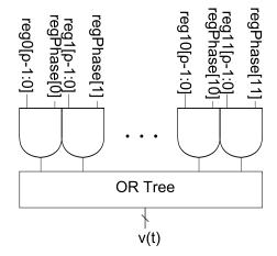
Figure 3.4: Parity output circuitry for the  $T_s = 192$ ,  $\rho = 16$ , rate-1/2 (3,6) PN-LDPC-CC, group period  $T'_s = 12$ . [1]
