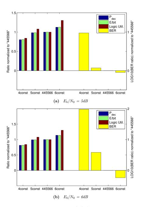
**Figure 6.5:** Decoder power, energy-per-coded-bit (E/bit), Logic Utilization, BER normalized to that of the "445566" case. The decoder power and energy-per-coded-bit values are based on the "mapped" values from the DC/DC converter efficiency experiment.
