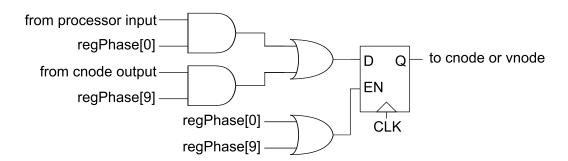
Figure 3.7: An example of a clock-gated register [1]
