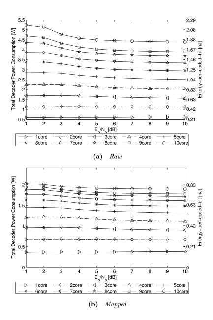
Figure 5.2: Average measured decoder power and energy-per-coded-bit at various  $E_b/N_0$  for various numbers of decoder cores on DE4 with 4-bit LLRs at a 75MHz clock with coded throughput of 2.4 Gbit/s for the  $T_s = 192$ ,  $\rho = 16$ , rate-1/2 (3,6) PN-LDPC-CC code based on three sets of measurements for each data point.
