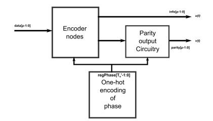
Figure 3.2: A high-level block diagram of the implemented PN-LDPC-CC encoder. An example of a single encoder node is shown in Figure 3.5. The one-hot encoding of the phase signal is shown in Figure 3.3. Figure 3.4 depicts the parity output circuitry.
