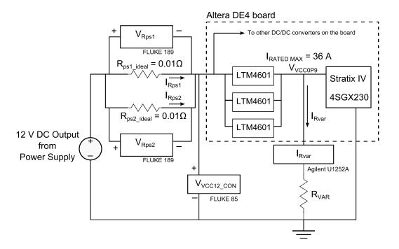
**Figure 4.4:** Schematic for DC/DC efficiency experiment
