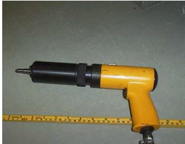
Figure 2.13: Pneumatic riveting gun used for hammer peening (Haagensen & Maddox, 2001)
