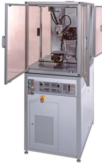
Figure 3.25: LXR residual stress measurement System (Proto. Manufacturing Ltd., 2011)
