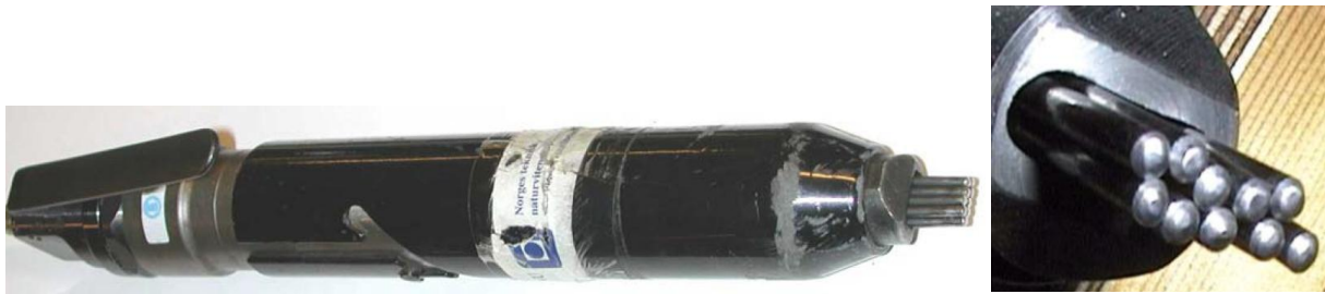
Figure 2.15: Needle peening equipment (left) and the tip (right) (Haagensen & Maddox, 2001)
