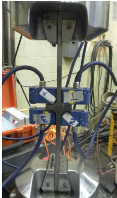
Figure 3.10: ACPD probes on the specimen in the machine
