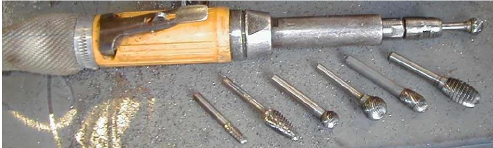
Figure 2.12: Grinder and burrs (Haagensen & Maddox, 2001)
