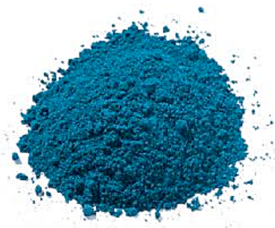
Figure 6. The specific blue colour of Prussian blue \text{Fe}^{\text{III}}_4[\text{Fe}^{\text{II}}(\text{CN})_6]_3 \cdot z\text{H}_2\text{O} .
