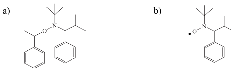
Figure 9.7 Structures of a) N-tert-butyl-N-(2-methyl-1-phenylpropyl)-O-(1-phenylethyl)hydroxylamine (TIPNO-based alkoxyamine), and b) 2,2,5-trimethyl-4-phenyl-3-azahexane-3-oxyle (TIPNO)
