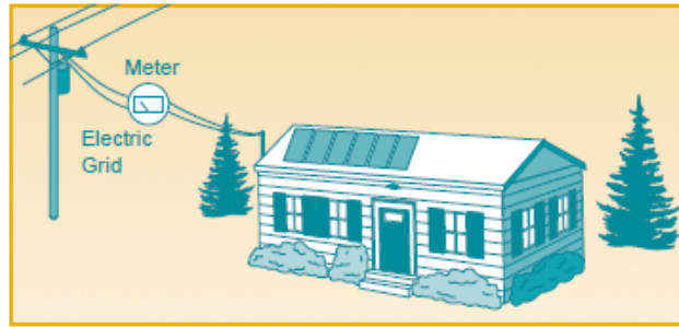
Fig. 1-3: Grid-connected PV system [1].
