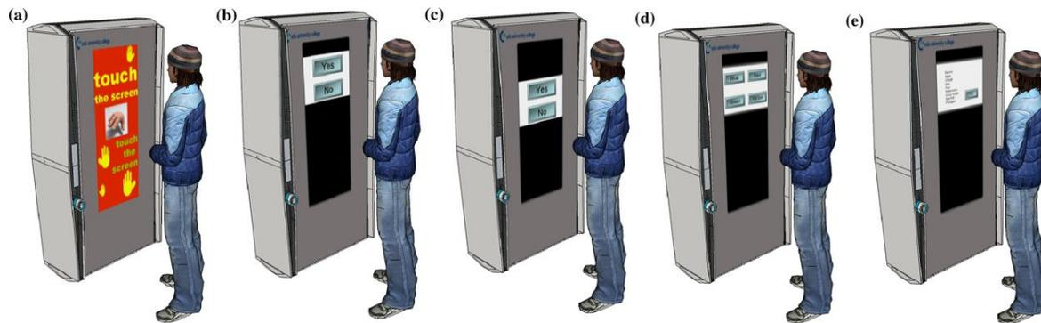
**Figure 2.5:** Dynamically altering the text size and center of interaction on a kiosk.
