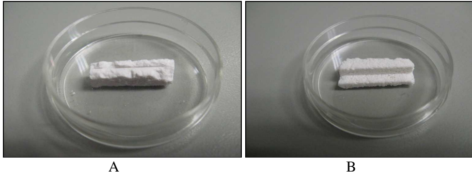
Figure 3-8: Comparison Images for Surface Integrity. A: Chipping along edges for Run #4; B: No Chipping Along Edges, Run #9.
