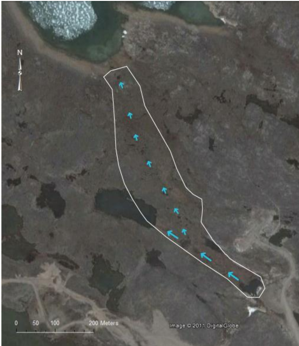
Figure 4. Aerial view of Chesterfield Inlet treatment wetland delineating wetland boundaries and flow directions.
