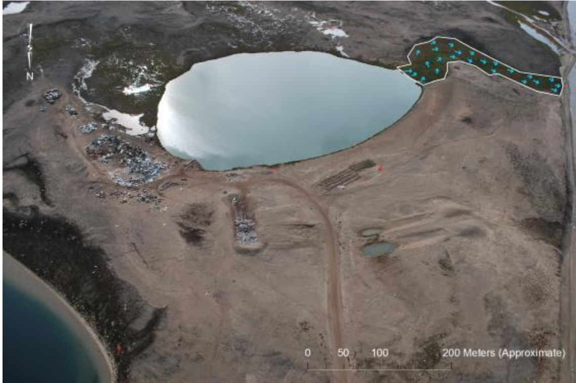
Figure 5. Aerial view of Paulatuk treatment wetland delineating wetland boundaries and flow directions (see top right of photograph).
