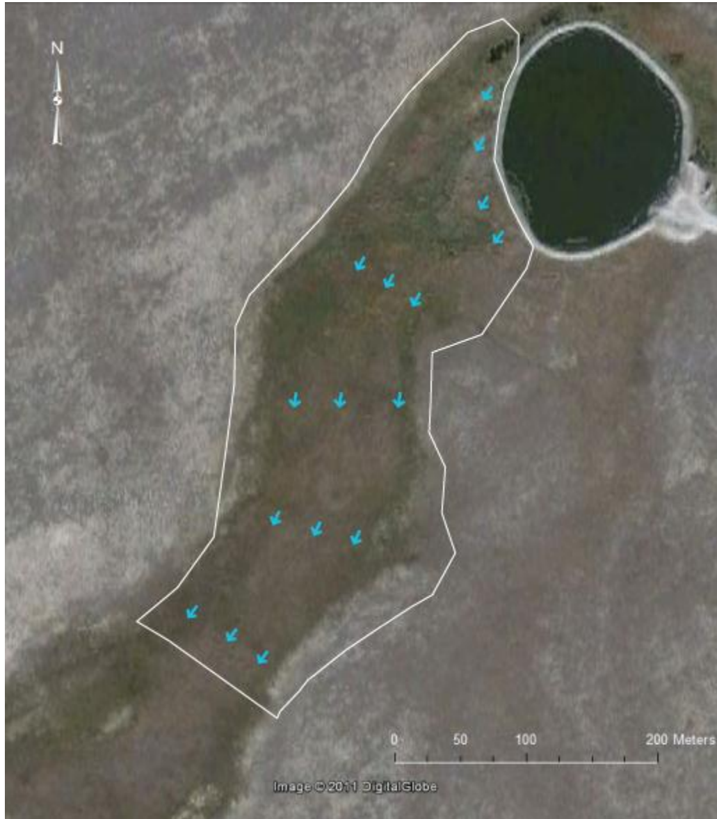
Figure 6. Aerial view of Uluhaktuk treatment wetland delineating wetland boundaries and flow directions.
