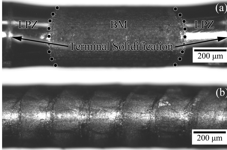
Figure 3.5: NiTi SMA wires processed at -55% OL (a) and 75% OL (b). Superficial bulging of the wire cross-section is evident along the terminal solidification front in (a).
