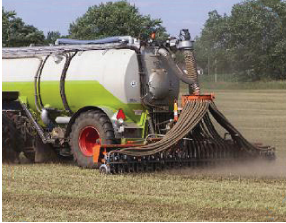
Fig 2.28 Equipment used to apply digestate to fields as a soil fortifier. In this application, the digestate is applied under pressure to inject it deep into the soil structure, maximizing the improvement to soil fertility
