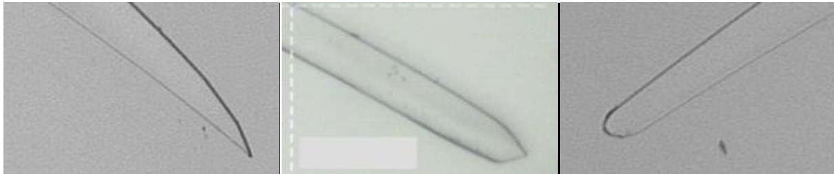
Figure 1-5: Contact lens/edge shapes: knife point (left), chisel (center) and round.
