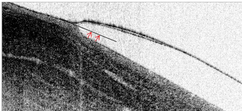
Figure 4-2: Soft contact lens edge on a continuous glass surface.
