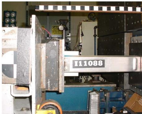
Figure 15: Fast Axial Crush Fixture [9]
