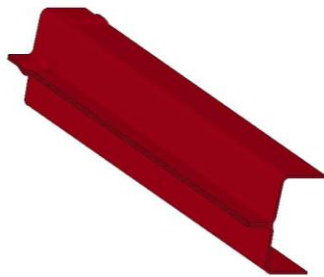
Figure 30: AM60 and AZ31 Crush Model
