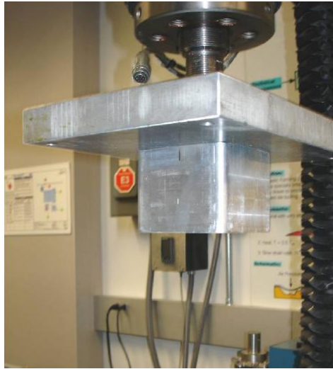
Figure 14: Slow Axial Crush Fixture [9]
