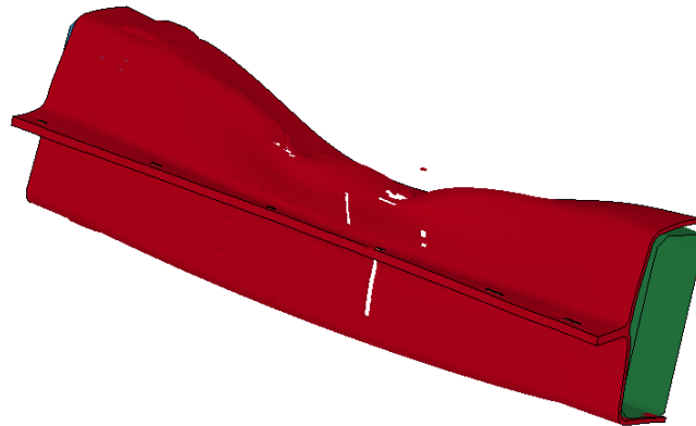
Figure 55 AZ31 Four Point Bend Test Crushed Tube with Rivets
