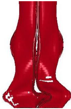
Figure 39: AZ31 Simulation Prediction Results (Fast Crush)
