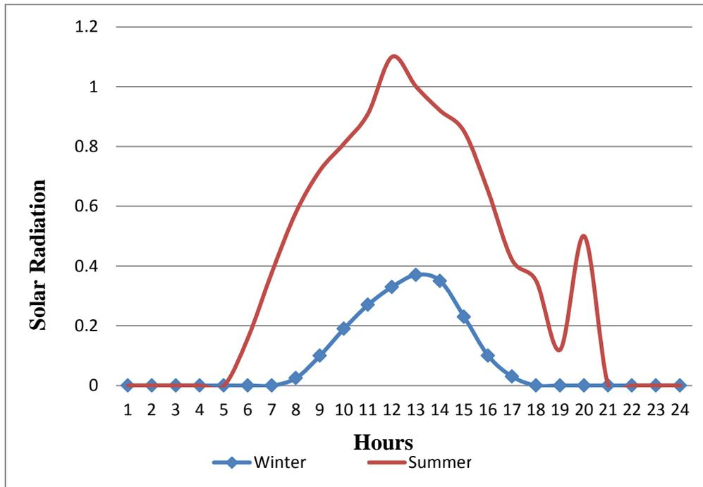
**Figure 4-4: Solar radiation profiles for winter and summer (kWh/m<sup>2</sup>)**
