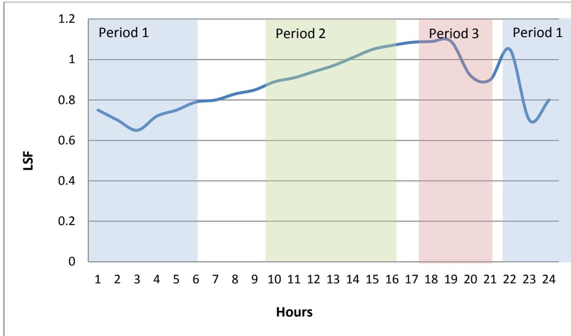
Figure 3-2: Load scale factors for the distribution system bus loads
