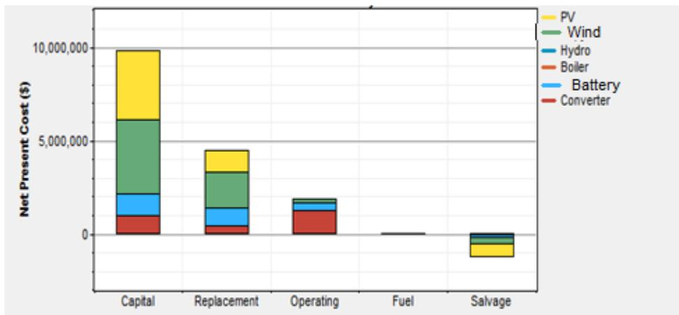
Figure 2-8: Cost components for Case-2 microgrid
