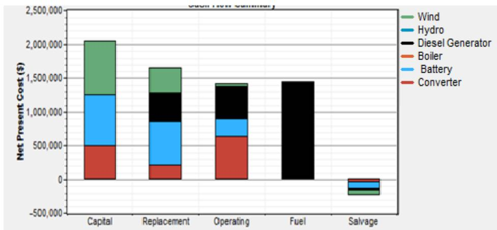
Figure 2-9: Cost components for Case-3 microgrid
