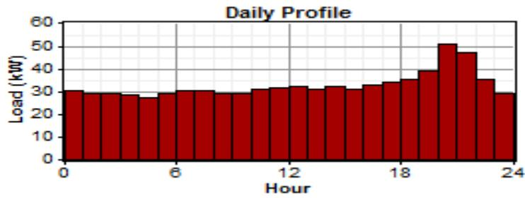
**Figure 2-3: Hourly electrical load profile of microgrid**
