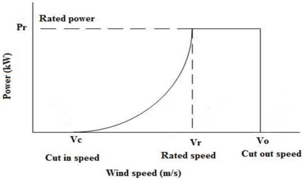
**Figure 4-1: Wind turbine ideal power curve [16]**
