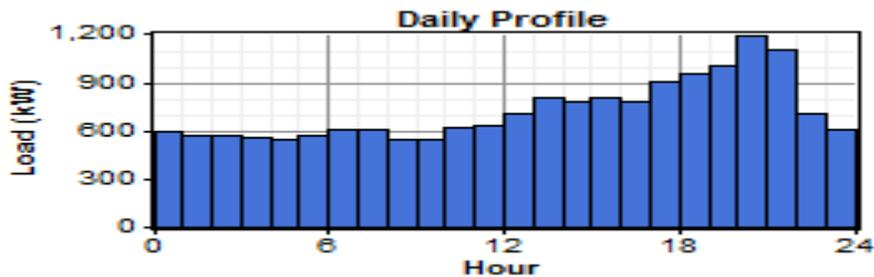
**Figure 2-2: Hourly electrical load profile of microgrid**
