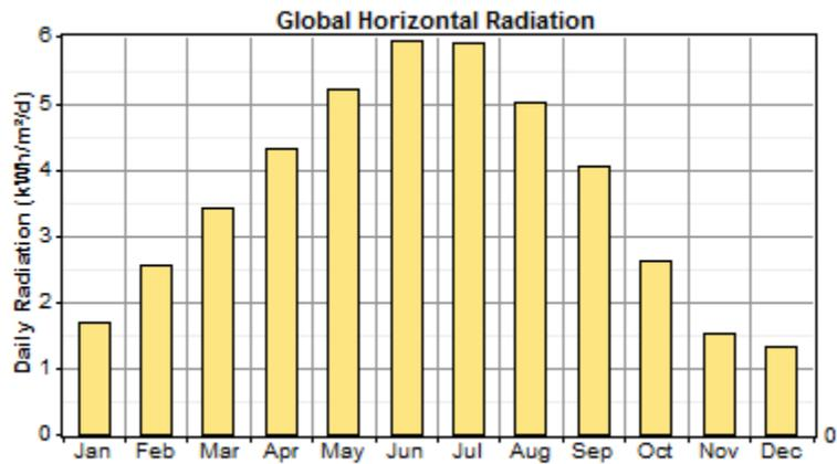
**Figure 2-4: Solar radiation profile for Waterloo**
