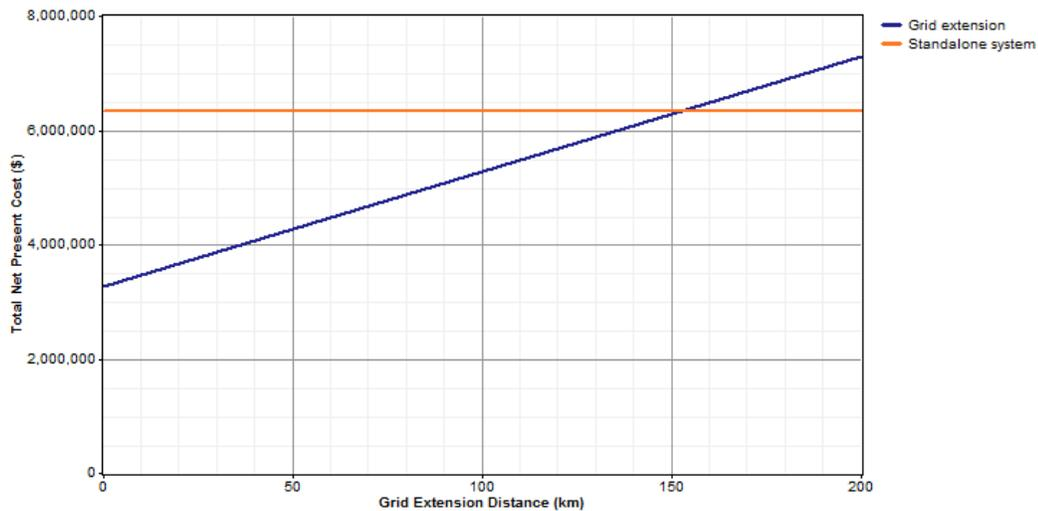
**Figure 2-19: Variation of NPC with grid connectivity distance for Case-3 microgrid**
