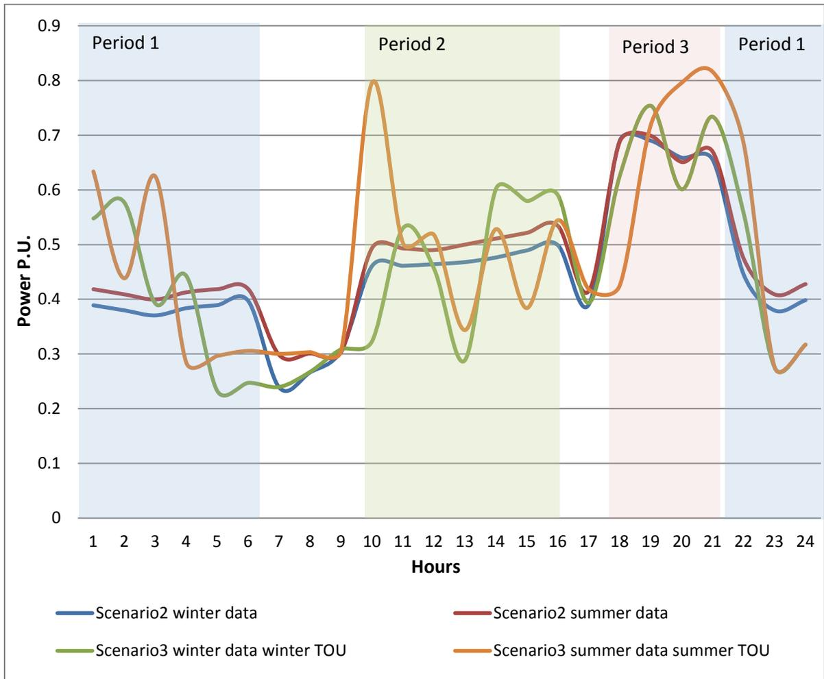
**Figure 4-11: Active power transfer over substation transformer**
