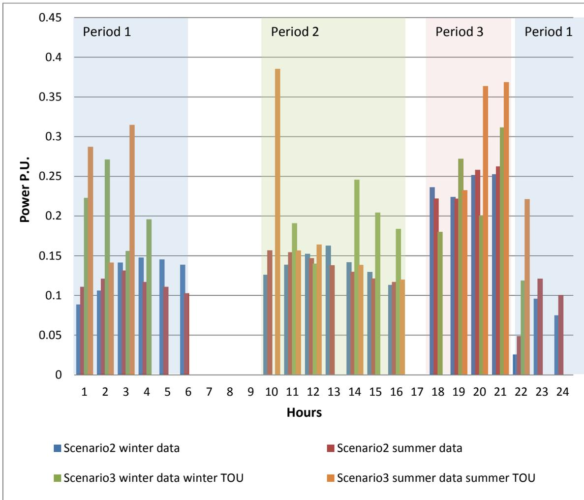
**Figure 4-7: Optimal charging profile of PHEV in different scenarios**
