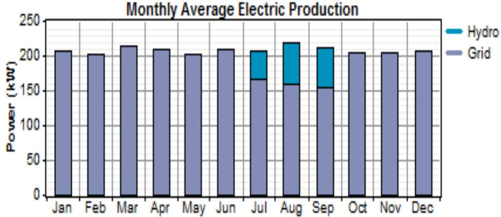
**Figure 2-17: Power production in Case-4 Microgrid**
