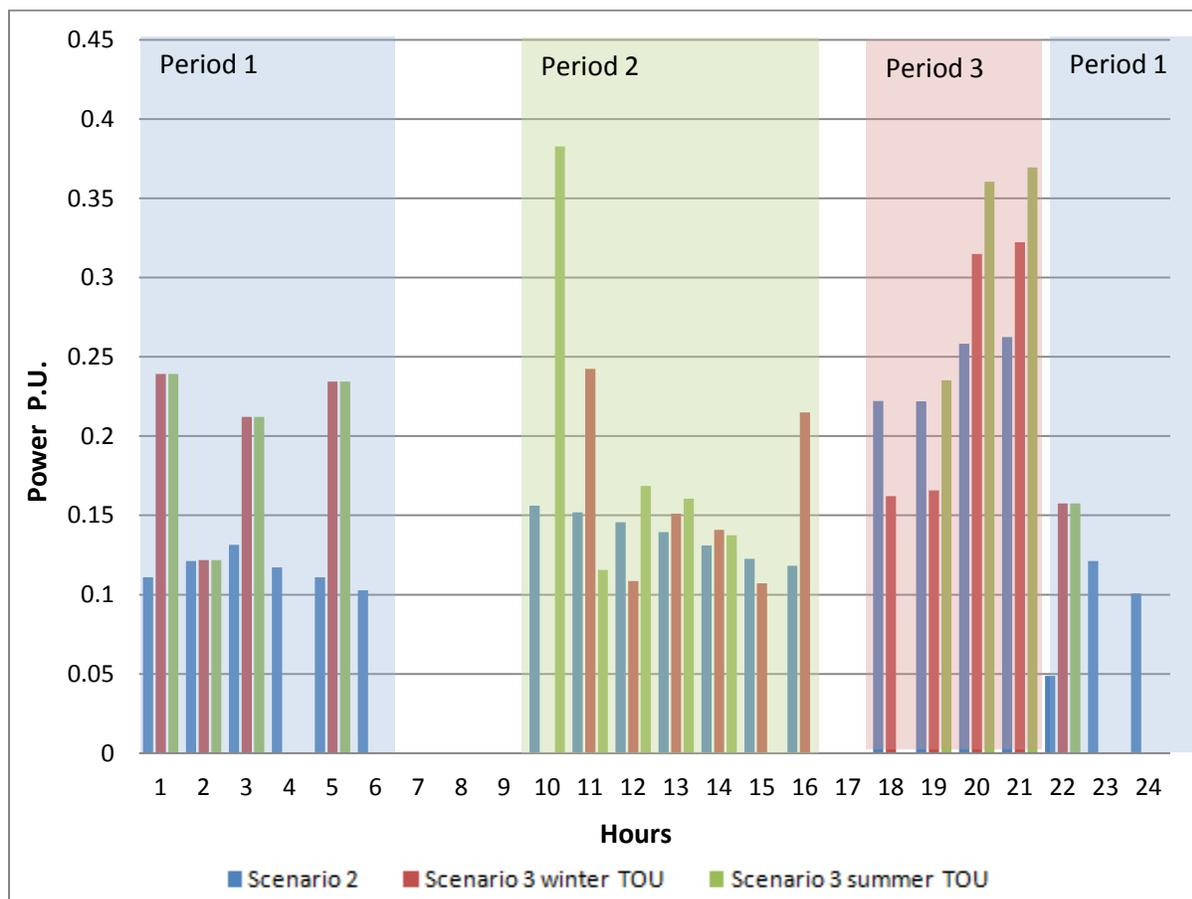
Figure 3-4: Optimal charging profile of PHEV in different scenarios
