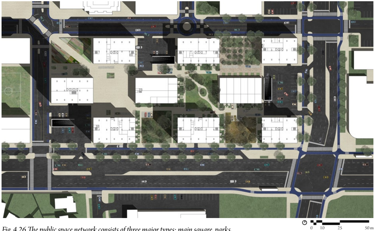
Fig. 4.26 The public space network consists of three major types: main square, parks, and service courts, distributed throughout each block
