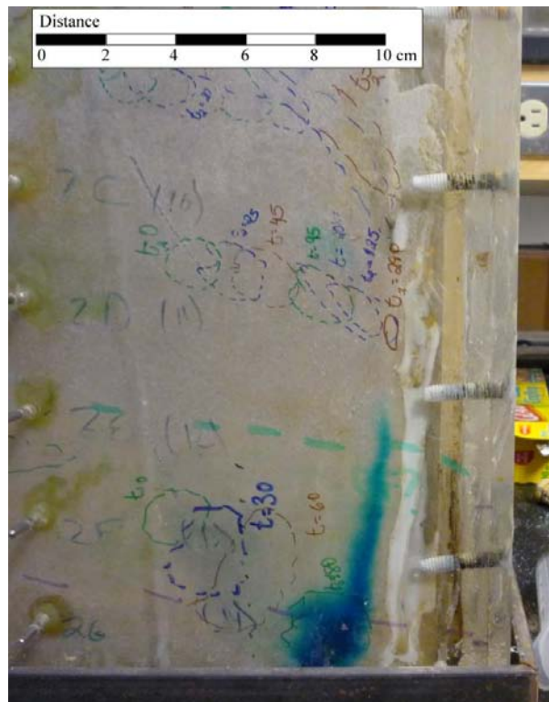
Figure 5.9. Saturated dye pulse flow near tank outlet.
