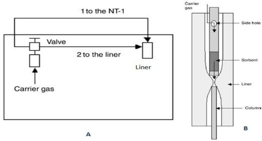
**Figure 1-3 Schematic illustration of A: Carrier gas diverting line; B: NTD inside the narrow neck liner during desorption [15]**
