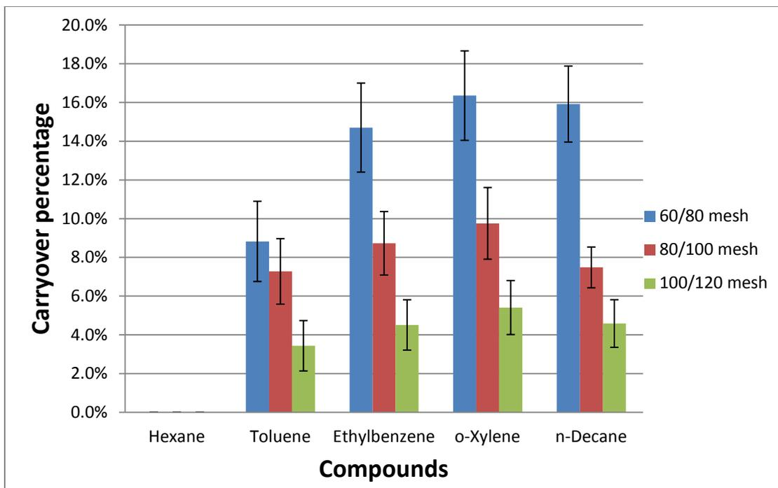
**Figure 4-2** Carryover percentages of NTDs packed with 1 cm DVB of different sizes with thermal expansion desorption (n=12: three needles, quadruplicate)
