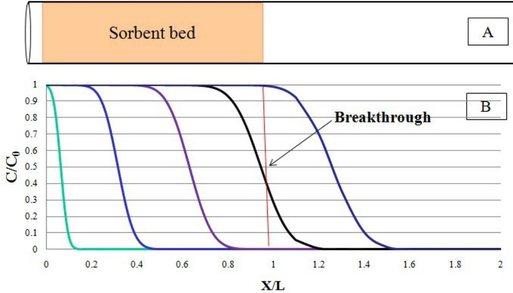
**Figure 1-5 A: Schematic representation of a packed needle; B: Theoretical concentration profiles in the sorbent bed, where  $C$  is the concentration of the analyte in the sample,  $L$  is the length of the sorbent bed,  $X$  is the relative position along  $L$ .**
