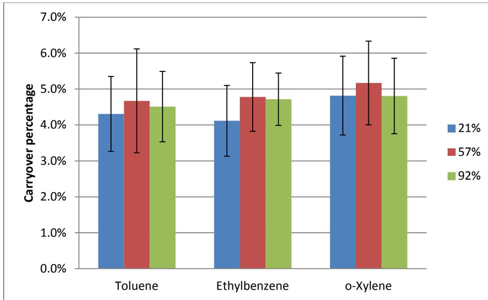
**Figure 4-8 Carryover percentages of DVB-NTDs with different humidities using thermal expansion desorption (n=8: two needles, quadruplicate)**
