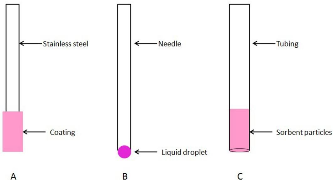
**Figure 1-1 Schematics of: (A) an SPME fibre; (B) an LPME extraction needle; (C) Sorbent trap.**
