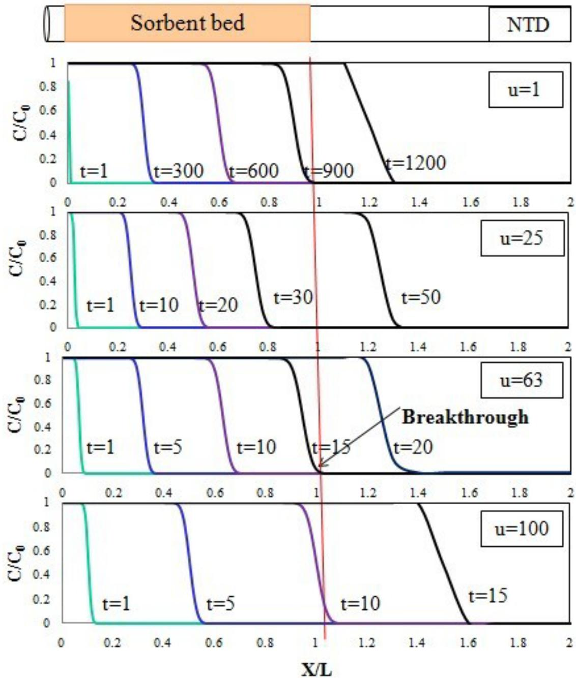
Figure 3-3 The concentration profile of the elution front along the  $x$ -axis at different time  $t$  (seconds) with different  $u$  (cm/s) ( $n=1000, k=1000$ )
