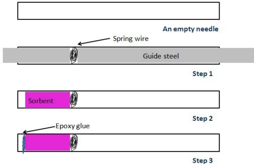
Figure 2-1 Schematic illustration of the packing procedure
