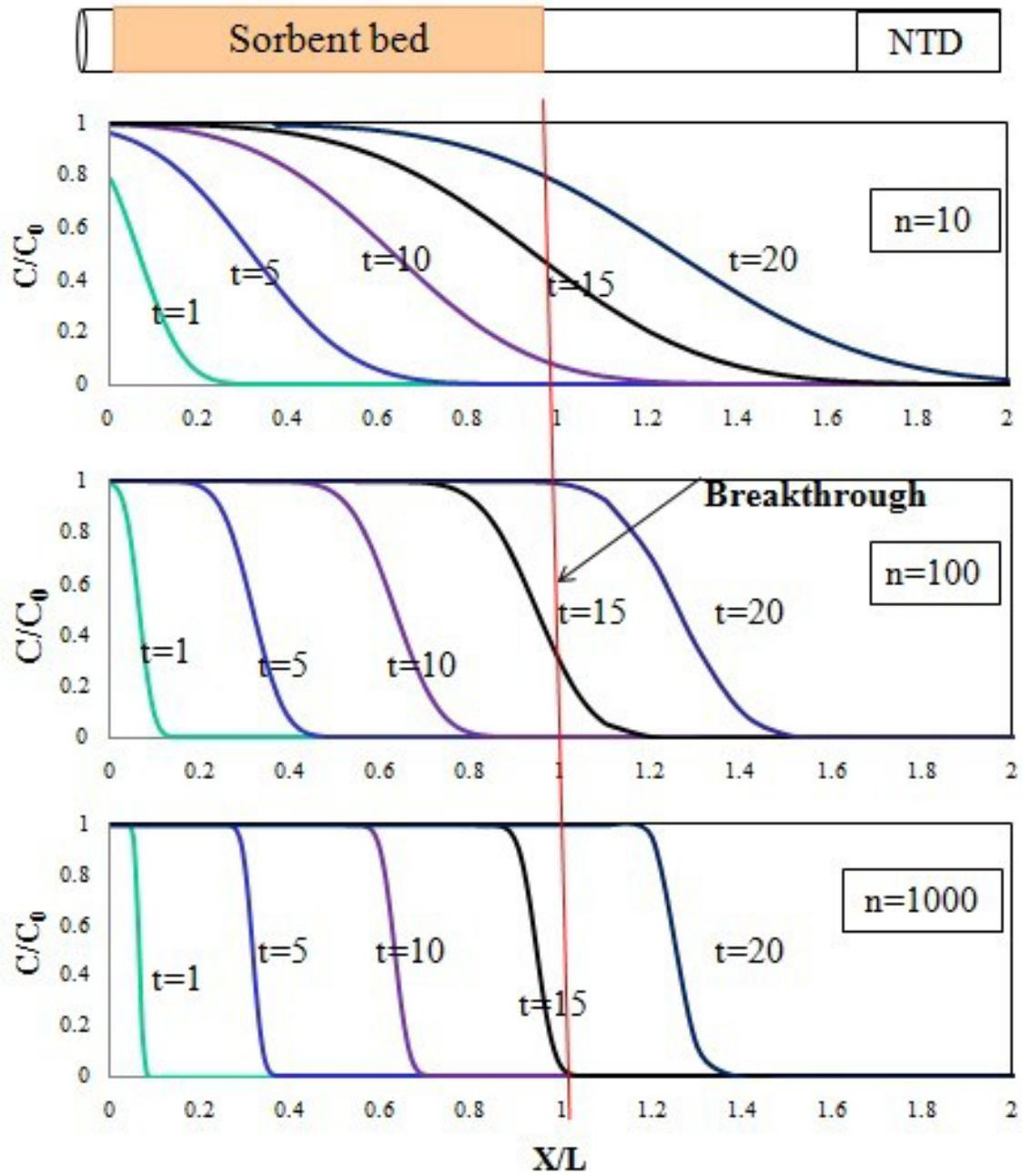
Figure 3-1 The concentration profile of the elution front along the  $x$ -axis at different time  $t$  (seconds) with different  $n$  ( $u=63$  cm/s,  $k=1000$ )
