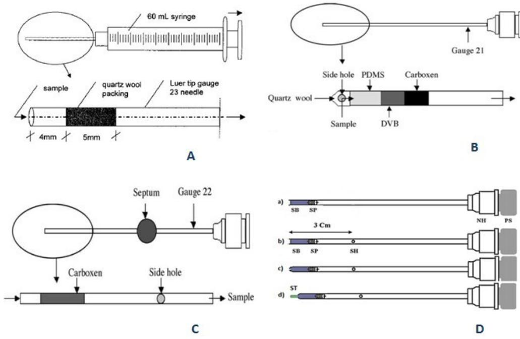
**Figure 1-2 Schematic illustration of the evolution of NTD designs in Pawliszyn’s group [14,15,16,17]: (A) a glass wool packed needle; (B) multi-sorbent beds needle; (C) a side hole needle; (D-a) a blunt tip non-side hole needle; (D-b) a blunt tip needle with a side hole; (D-c) a conical tip needle with a side hole; (D-d) an extended tip needle with a side hole**
