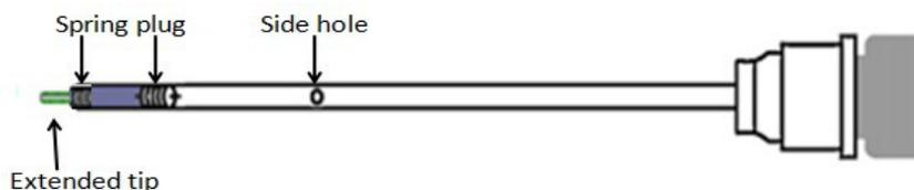
**Figure 5-2 Schematic diagram of a packed needle**
