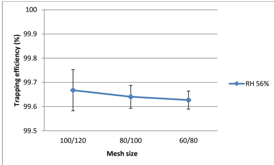
Figure 5-4 Collection efficiencies of NTDs packed with DVB of 60/80 mesh, 80/100 mesh and 100/120 mesh (n=4: two needles, duplicate for each needle.)
