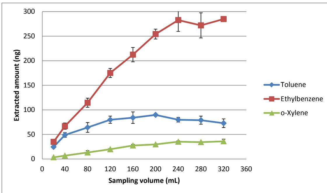
**Figure 3-5 Breakthrough volumes of TEX compounds using NTDs packed with 60/80 mesh Tenax GC (n=4, two needles, duplicate for each needle)**
