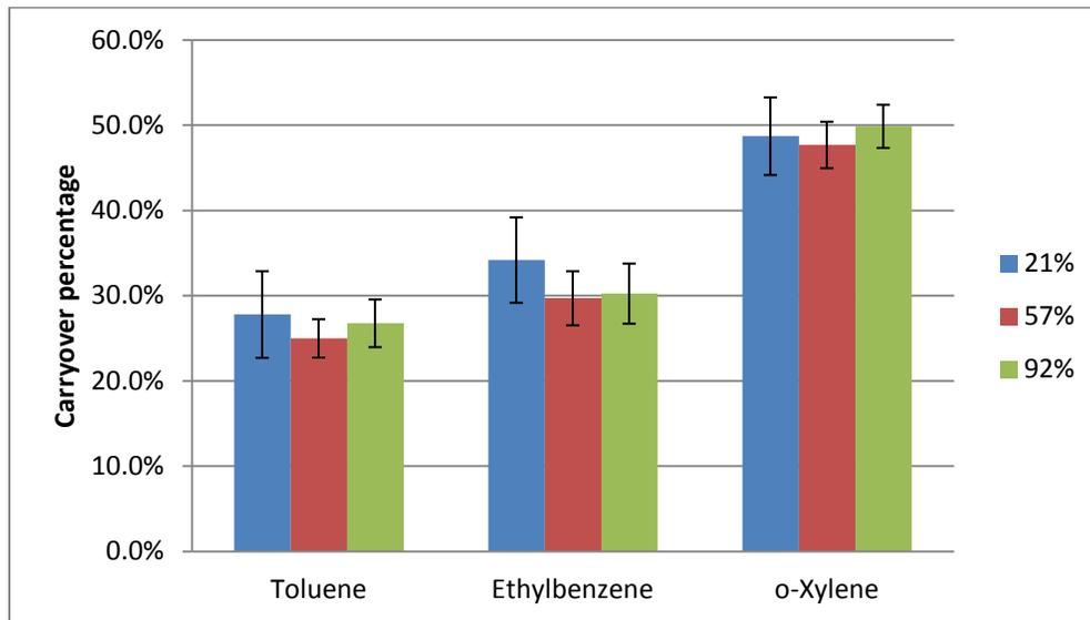
**Figure 4-9 Carryover percentages of CAR-NTDs with different humidities using thermal expansion desorption (n=8: two needles, quadruplicate)**
