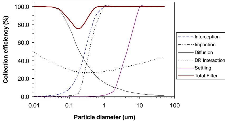
**Figure 1-7 Illustration of collection efficiency for individual single-sorbent mechanisms and total efficiency;  $L=1\text{ mm}$ ,  $\alpha=0.05$ ,  $d_p=2\mu\text{m}$  and  $u=10\text{ cm/s}$  [45]**
