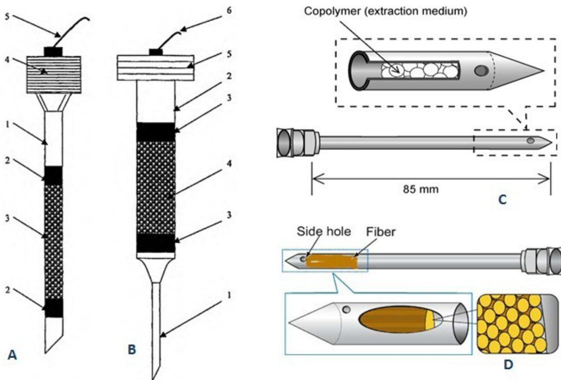
**Figure 1-4 Schematic illustration of (A) Needle microconcentrator: 1-needle stem; 2 plugs, limiting the sorbent layer; 3-sorbent layer; 4-holder; and 5-capillary line for carrier gas. (B) Cylindrical microconcentrator: 1-needle stem; 2-tube stem; 3-plugs, limiting the sorbent layer; 4-sorbent layer; 5-holder; and 6-capillary line for carrier gas. (C) Copolymer particles packed needle. D: Polymer coated fibre packed needle [18,19].**
