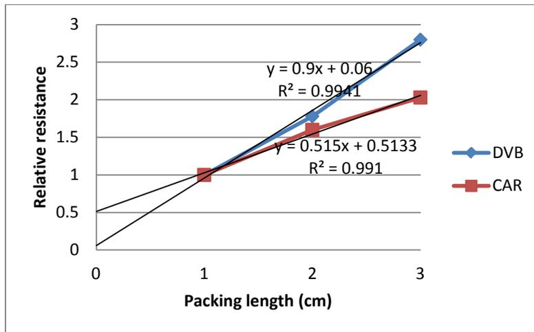
**Figure 2-2 Schematic illustration of the relative resistance with the increase of packing length for DVB and CAR needles**
