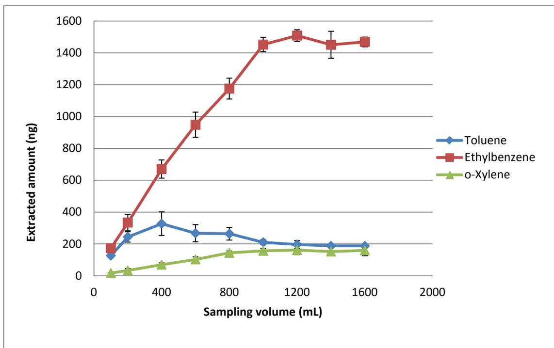
Figure 3-4 The breakthrough volumes of TEX compounds using NTDs packed with 60/80 mesh DVB (n=4: two needles, duplicate for each needle)
