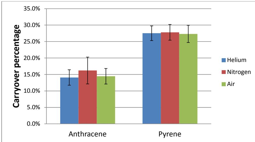
**Figure 4-6 Carryover percentages of DVB-NTDs with different external gas assisted desorption (n=8: two needles, quadruplicate)**
