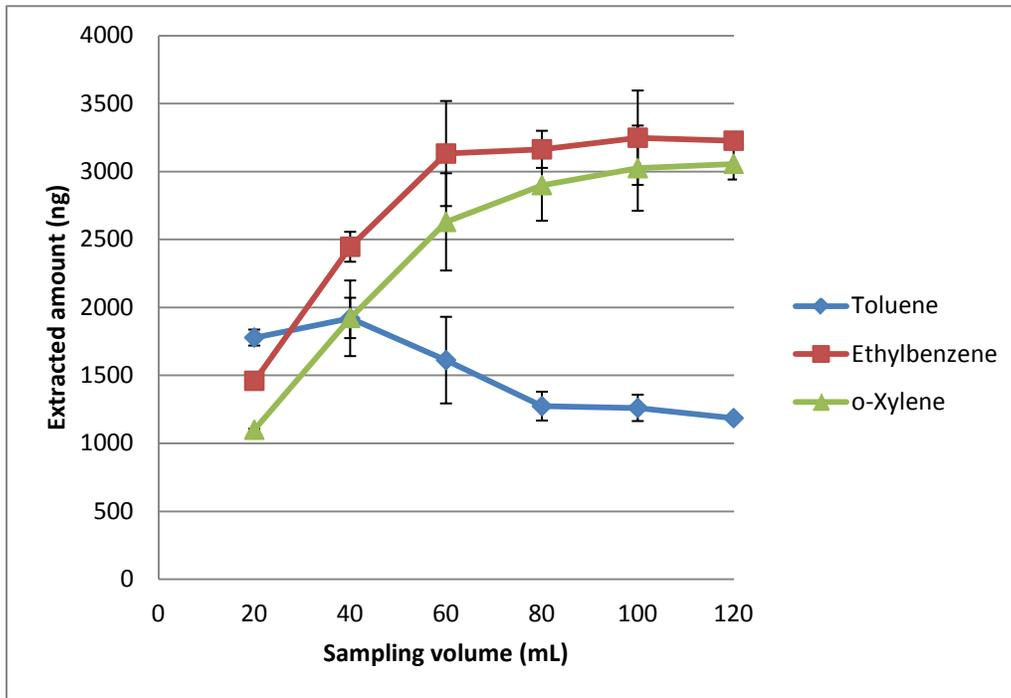
**Figure 3-6 Breakthrough volumes of TEX compounds at high concentrations using NTDs packed with 60/80 mesh DVB (n=4, two needles, duplicate for each needle)**
