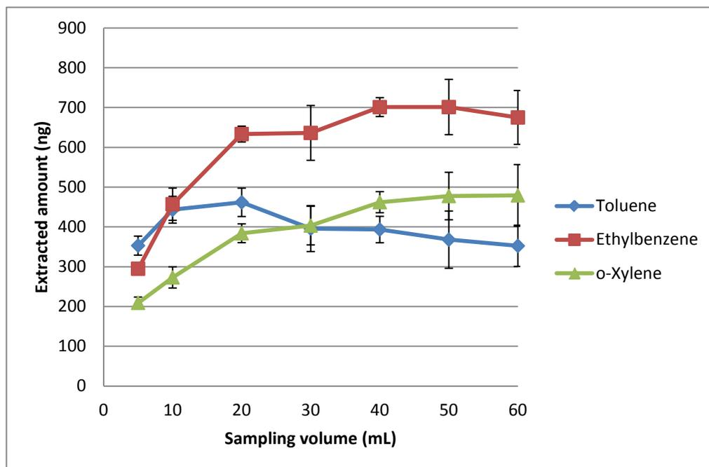
**Figure 3-7 Breakthrough volumes of TEX compounds at high concentrations using NTDs packed with 60/80 mesh Tenax GC (n=4, two needles, duplicate for each needle)**
