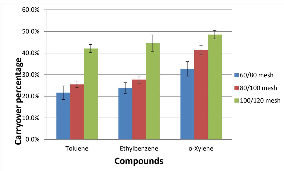
**Figure 4-3** Carryover percentages of NTDs packed with 1 cm CAR of different sizes with thermal expansion desorption (n=8: two needles, quadruplicate)
