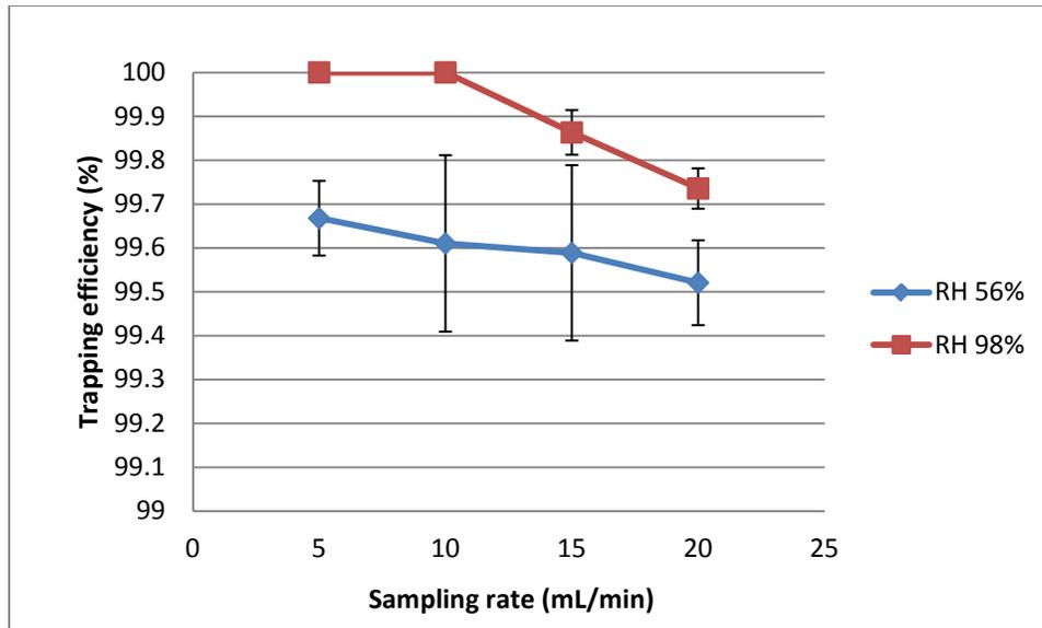
**Figure 5-5** Collection efficiencies of NTDs packed with 100/120 mesh DVB under different sampling rates and different humidity levels (n=6: two needles, triplicate for each needle.)
