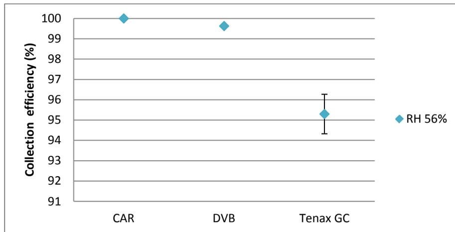
**Figure 5-3 Collection efficiencies of NTDs packed with different sorbent particles of 60/80 mesh (n=4: two needles, duplicate for each needle.)**
