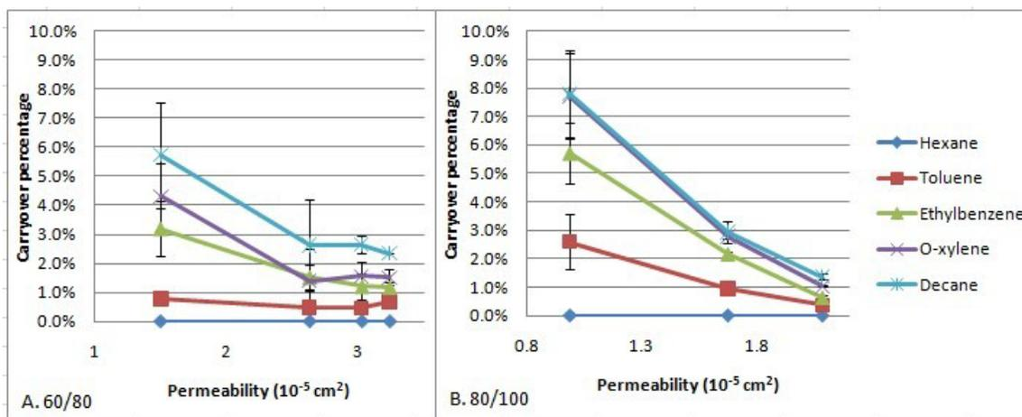
**Figure 4-1 Carryover percentages of different types of NTDs with different permeabilities**
