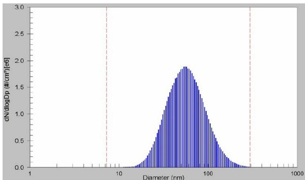
**Figure 5-1 Particle size and distribution of a sodium chloride aerosol generated from 0.1 mg/cm<sup>2</sup> solution [50]**
