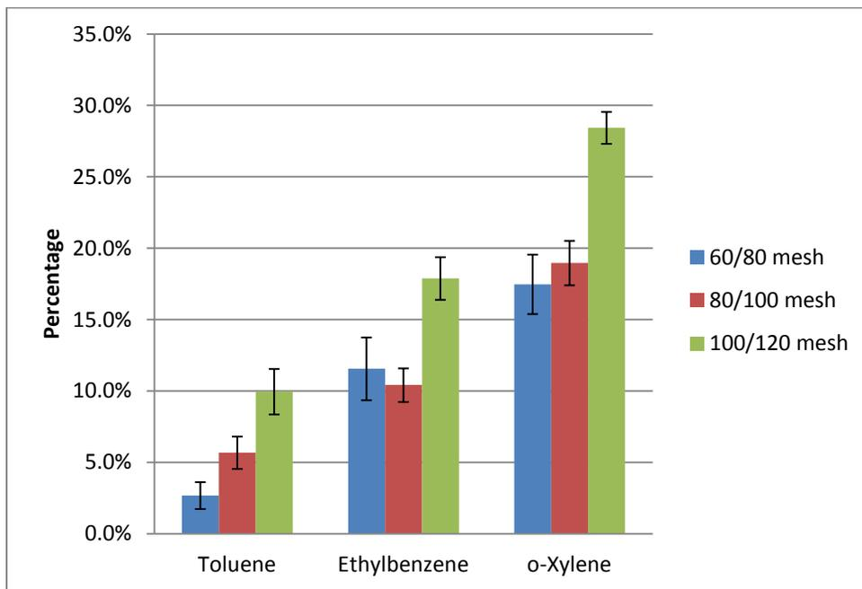
**Figure 4-5 Carryover percentages of NTDs packed with 1 cm CAR of different sizes with carrier gas assisted desorption (n=8: two needles, quadruplicate)**
