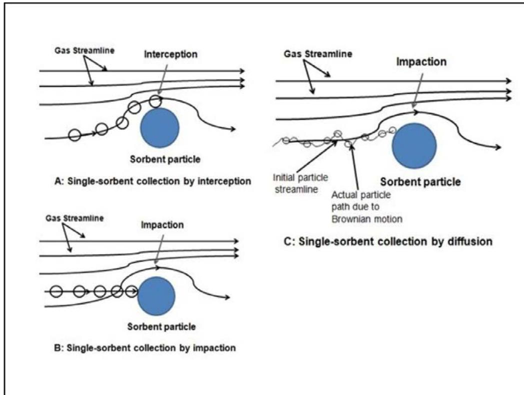
**Figure 1-6 Schematic explanation of interception, impaction, and diffusion [5]**
