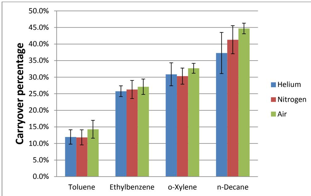
**Figure 4-7 Carryover percentages of CAR-NTDs with different carrier gas assisted desorption (n=8: two needles, quadruplicate)**
