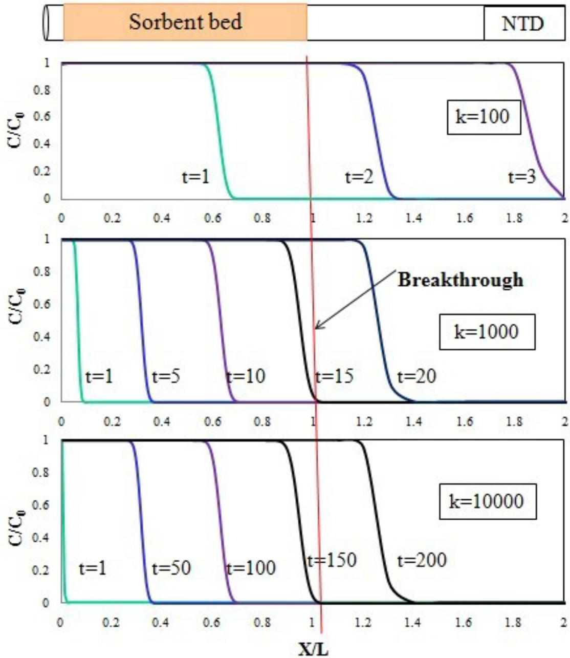
Figure 3-2 The concentration profile of the elution front along the  $x$ -axis at different time  $t$  (seconds) with different  $k$  ( $u=63$  cm/s,  $n=1000$ )
