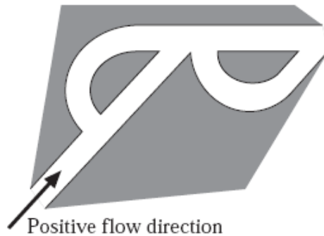
Figure 3-1: Non-mechanical Valvular Conduit Design for the Numerical Approach [29]
