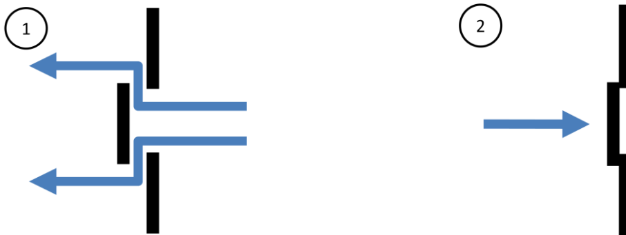
Figure 2-11: Schematics of Mechanical Check Valve – (1) Forward Flow; (2) Reverse Flow
