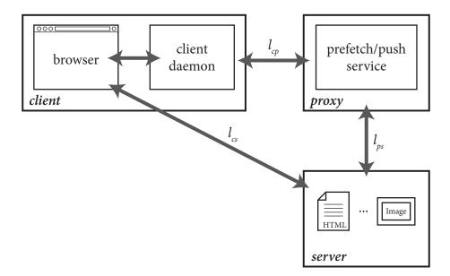
Figure 4.10: Additional path latency encountered in 3G test architecture
