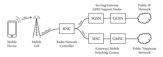
Figure 2.1: Detailed 3G network diagram
