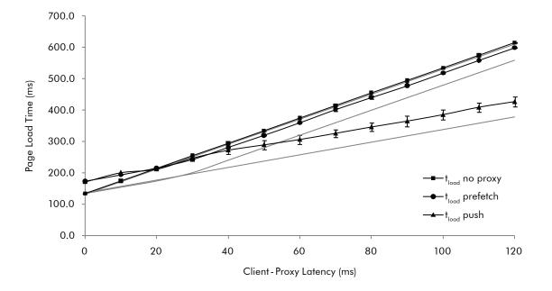
Figure 4.3: Actual load time for validation page with 1 embedded resource
