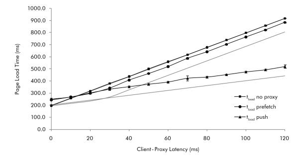
Figure 4.6: Actual load time for validation page with embedded resources to depth 2
