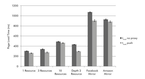
Figure 4.12: Load time for validation pages accessed using 3G data stick
