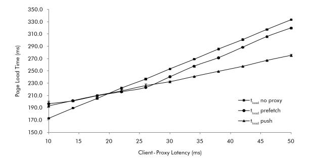
Figure 4.4: Actual load time for validation page with 1 embedded resource, 10–50 ms the characteristic change in slope occurring around  $l_{cp}$  = 30 ms, confirming our analysis.
