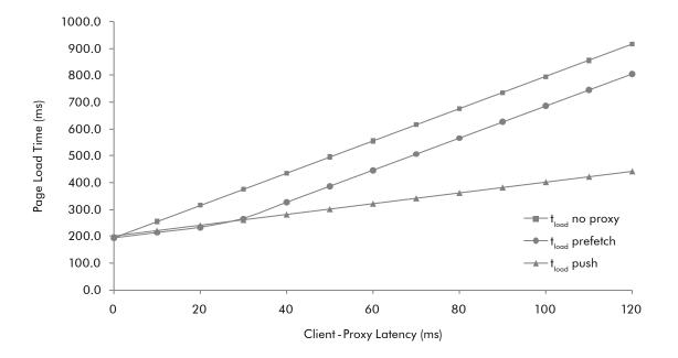
Figure 3.8: Total load time for page with embedded resources to depth 2
