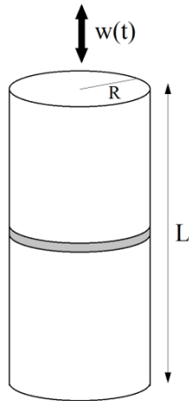
Figure 5-5- A rod with a central butt joint under cyclic loading
