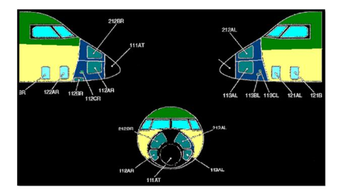
Figure A.6: Flight compartment subassembly: Physical layout and division of work areas
