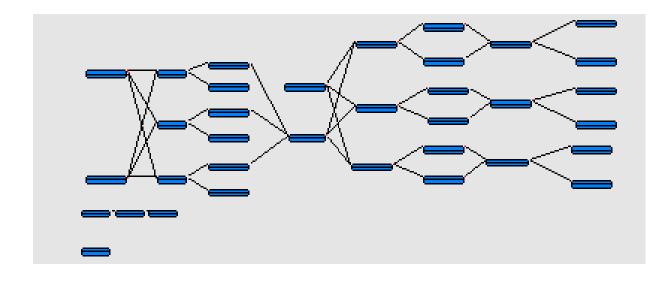
Figure A.3: Precedence relationship of operations in flight compartment work center
