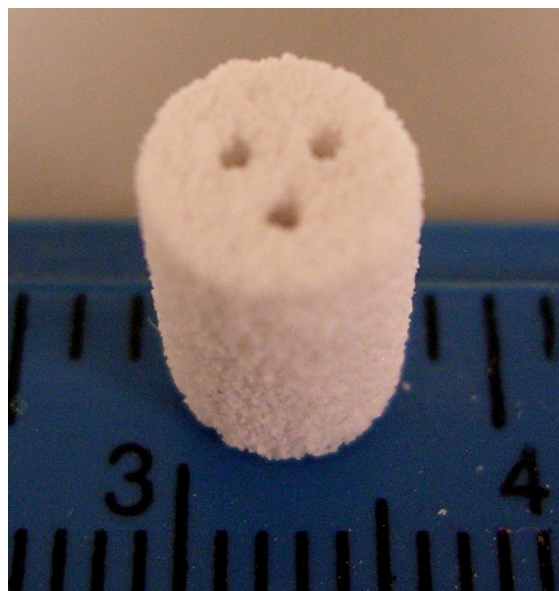
Figure 2-14: A randomly selected SFF-made CPP cylinder with 3 longitudinal channels.
