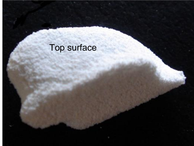
Figure 2-12: Fabricated medial portion of tibial plateau-shaped CPP structure; the top surface is intended for in vitro cartilage formation while bone ingrowth into the other surfaces allowing implant fixation to subchondral bone.
