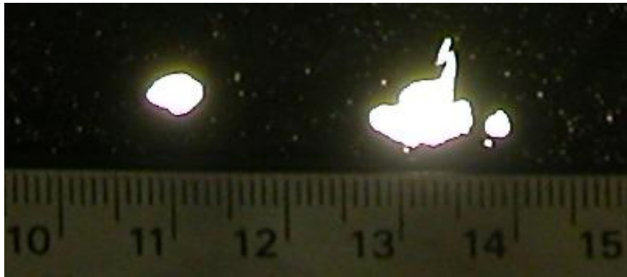
Figure 0-22: Freeze start-up cycled MEA focusing on formed pinhole
