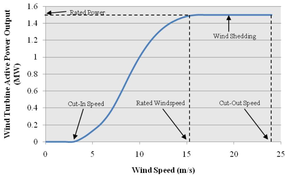
**Figure 2-9: Ideal Wind Turbine Power Curve.**
