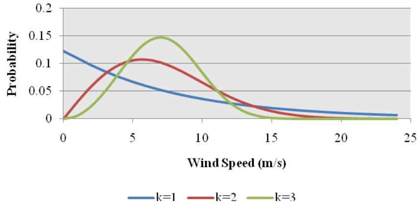
**Figure 2-7: Weibull PDF with Different Shape Parameter (k).**
