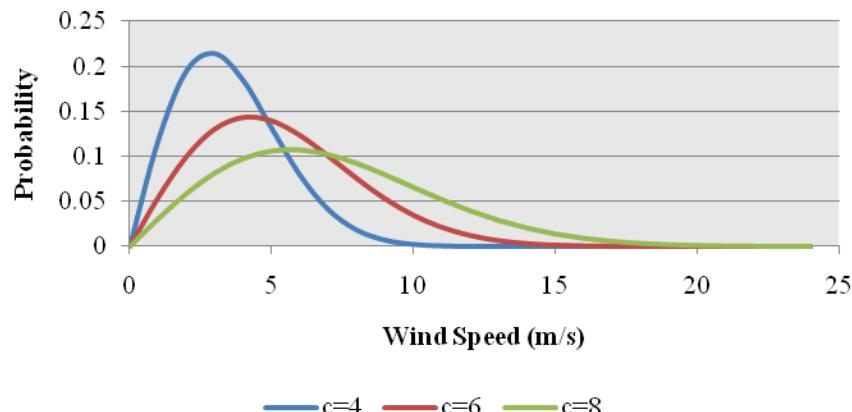
**Figure 2-8: Rayleigh PDF with Varying Scale Parameter (c).**
