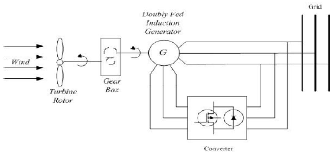
**Figure 2-5: Type C - Variable Speed Wind Turbines with Partial Scale Frequency Converters [19].**
