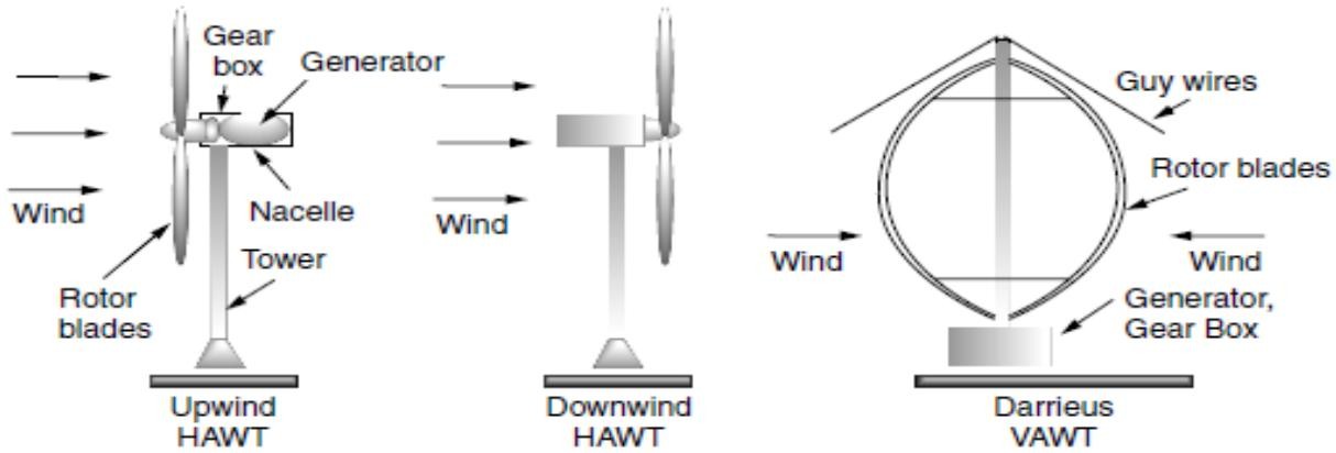
**Figure 2-2: Types of Wind Turbines [17].**
