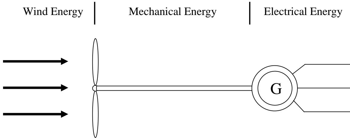
**Figure 2-1: Simplified Wind Generation Process.**
