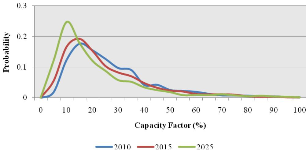
**Figure 4-12: PDF of Monte Carlo Simulation's Wind Generation's CF output (2010-2025).**
