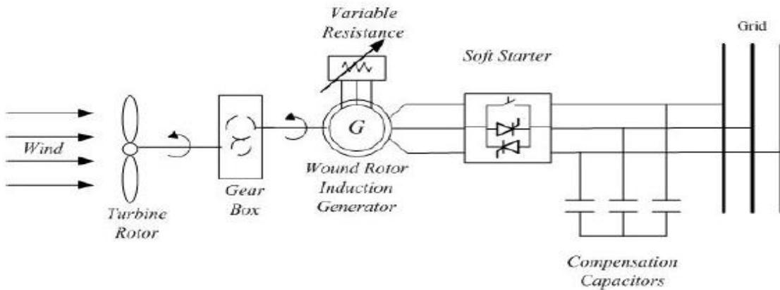
**Figure 2-4: Type B - Limited Variable Speed Wind Turbines [19].**
