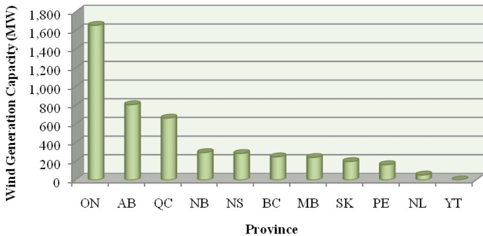
**Figure1-4: Canada’s Current Installed Wind Generation Capacity [2].**
