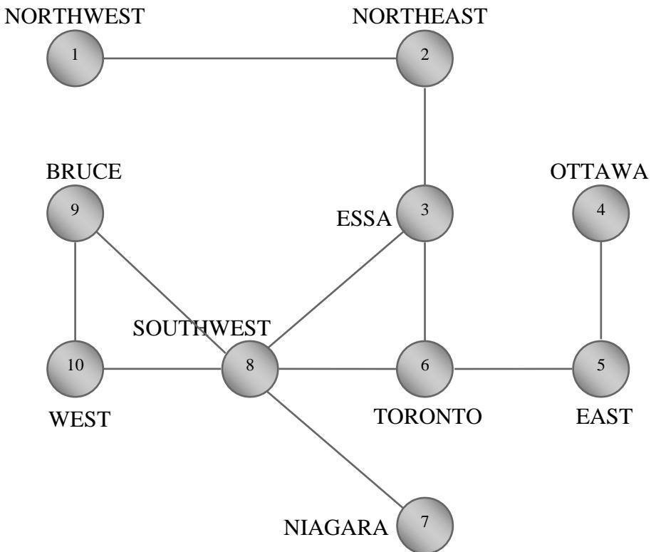
**Figure 4-1: Simplified Ontario Transmission Network.**
